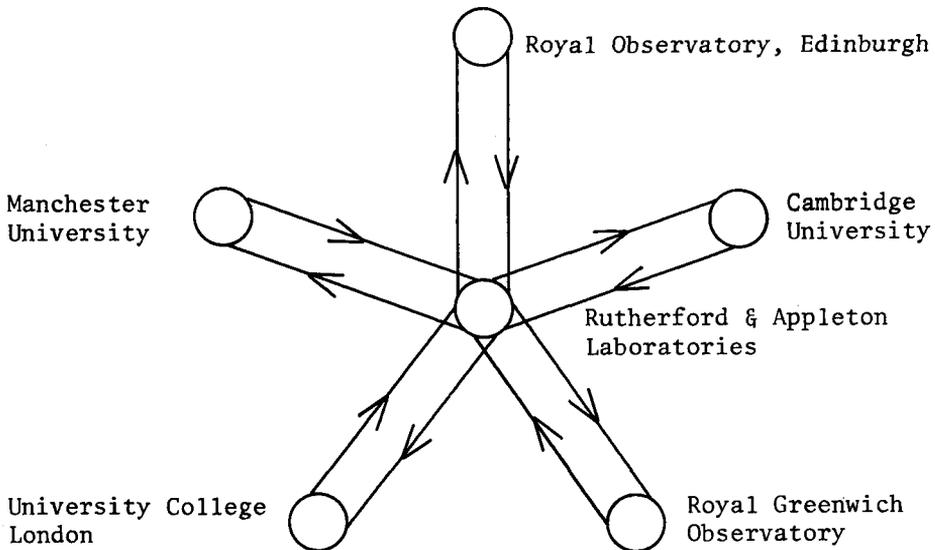
The transfer of data between sites has to go through the RAL node. Thus RAL can communicate directly with the other five computers, and vice-versa. But ROE can only communicate with RGO by following the path ROE - RAL - RGO. The system used to link the computers together is DECnet which is a product of Digital Equipment Corporation (DEC) who make the VAX computers.
