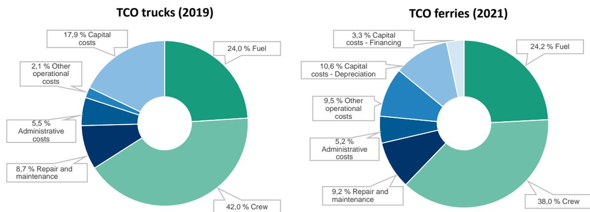
**Figure 1. TCO for domestic sea transport by ferries and trucks in the United States of America ([Almaas et al., 2021](#); [Williams and Murray, 2020](#))**
