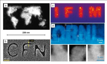
Figure 4. Examples of electron-beam-based fabrication. (a) Scanning transmission electron microscope image of a nanoscale topographic map of the world drawn using electronbeam-induced deposition and a tungsten precursor. Adapted with permission from Reference 77. © 2008 World Scientific. (b) Aberration-corrected electron-beam lithography in poly(methyl methacrylate).78 (c) IFIM. (d) Text "ORNL" patterned on the interface of amorphous and crystalline SrTiO<sub>3</sub>.79
