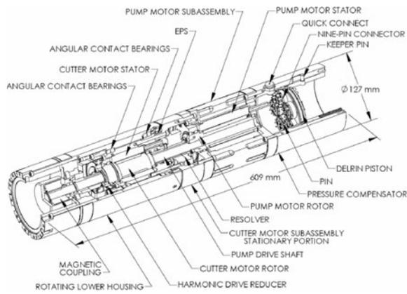
Fig. 3. Motor section.
