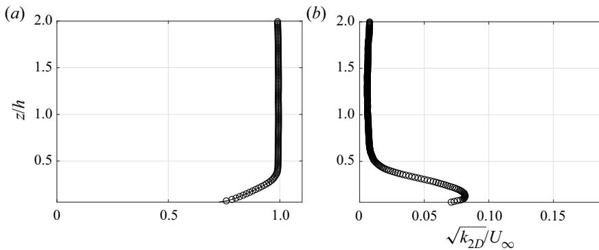
**Figure 3.** Background profiles of (a) the streamwise velocity and (b) turbulent kinetic energy (two-dimensional) both normalized by  $U_\infty$ . Note, these profiles are averaged over  $0.2h$  in the streamwise direction  $2h$  upstream of the leading edge of the first cube.
