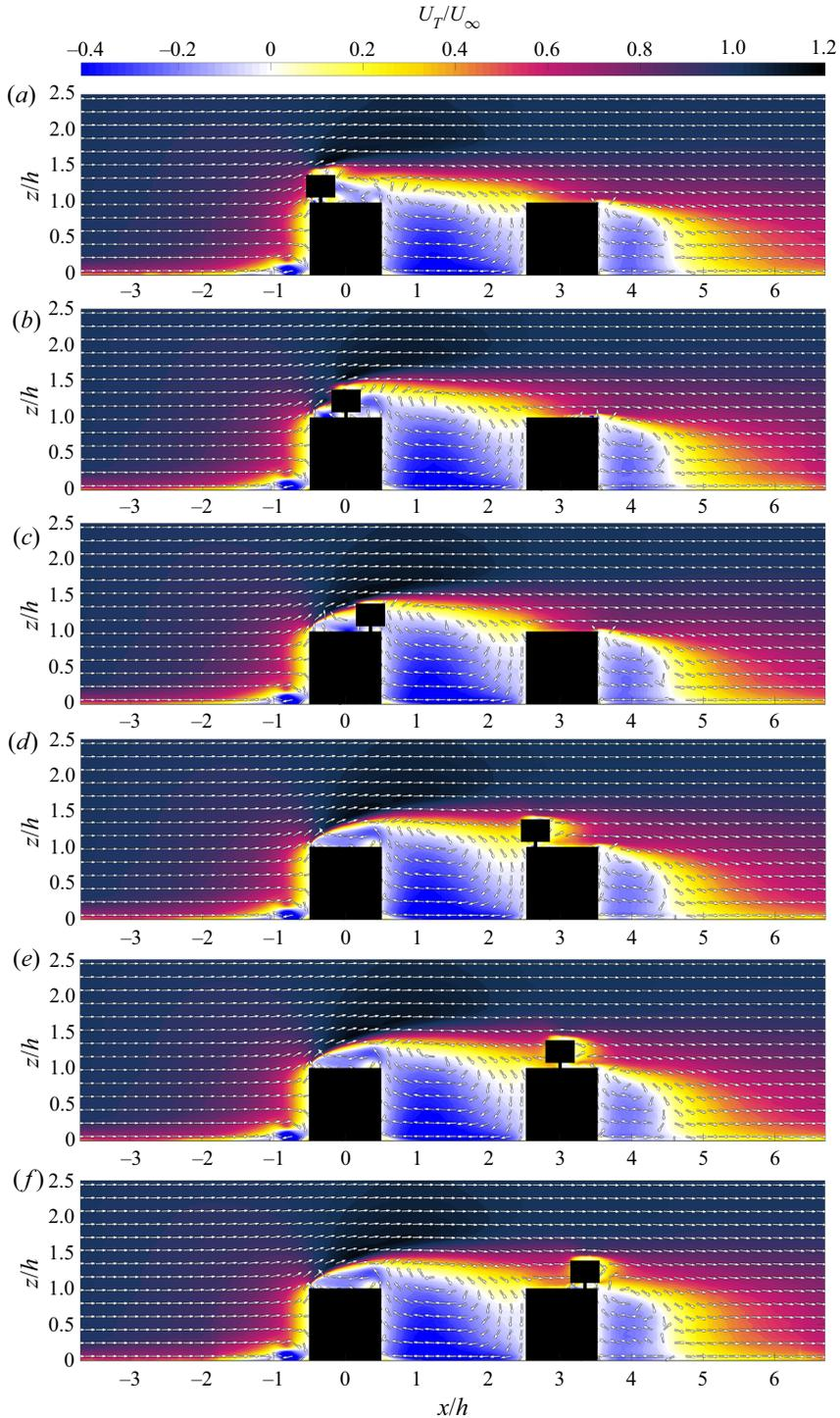
**Figure 6.** Streamwise velocity fields with the wind turbine mounted at different streamwise positions along the centreline. Note that only every 20th vector is displayed to avoid clutter and all velocity vectors are scaled to be of uniform length, only representing the direction of flow.
