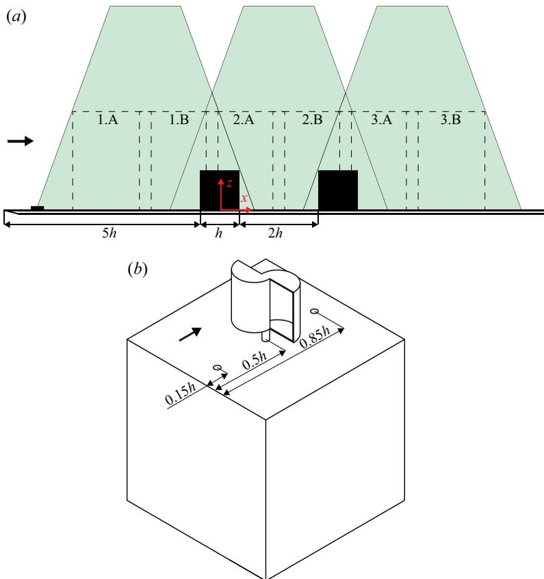
**Figure 1.** (a) Schematic of the experimental set-up. The flow fields were acquired in three separate acquisitions with two cameras (A and B). (b) The wind turbine was placed at three different positions along the centreline on each cube.
