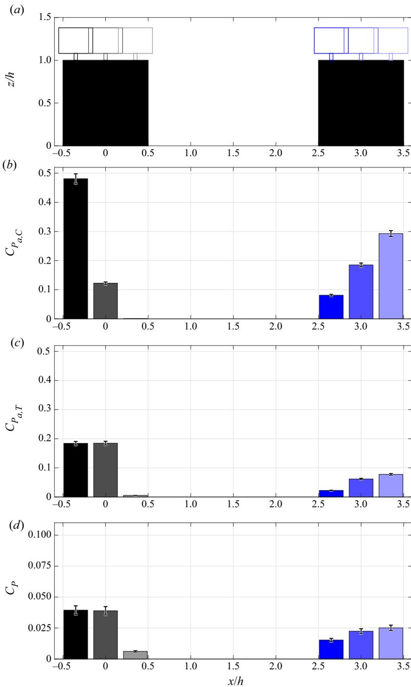
**Figure 9.** Analysis of the wind turbine performance at different positions based on the available power with and without the turbine ( $C_{P_{a,T}}$  and  $C_{P_{a,C}}$ ) and the measured mechanical power ( $C_P$ ). Uncertainty bars based on propagation of uncertainty of all contributing variables.
