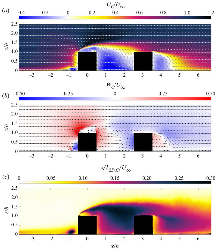
**Figure 4.** (a) Streamwise velocity, (b) wall-normal velocity and (c) turbulent kinetic energy fields normalized by  $U_\infty$  around the cubes without the turbine. Note that only every 20th vector is displayed to avoid clutter and all velocity vectors are scaled to be of uniform length, only representing the direction of flow.
