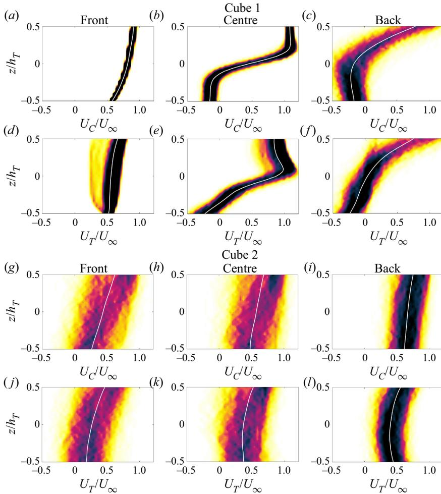
**Figure 8.** Histograms of streamwise velocity  $U$  along the turbine blade immediately ( $0.05d_T$ ) upstream of the turbine from the flow fields without ((a–c) and (g–i)) and with the turbine ((d–f) and (j–l)). Mean velocity profiles superimposed as white lines.
