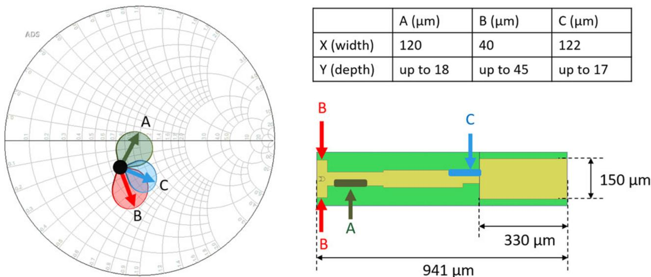
**Fig. 3.** Effect of trimming different areas on the WG-MS transition. The black dot on the Smith chart shows the initial measured  $S_{22}$  of the LNA, at the band center, 183.3 GHz. The letters A, B, and C show different trim areas on the circuit, and the corresponding arrows and shaded regions on the Smith chart show the direction of movement of the impedance as the conductor was removed.
