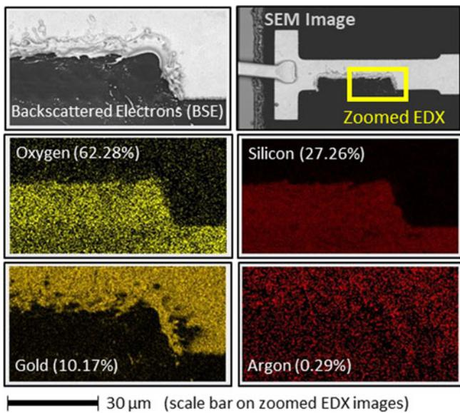
**Fig. 5.** EDX element map and atom abundance of a corner within the trimmed area of the transition.
