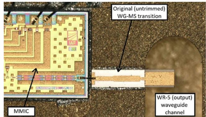
Fig. 1. Original untrimmed WG-MS transition assembled onto a 183 GHz LNA. The quartz dimensions are  $941 \times 200 \times 25$   $\mu\text{m}$ . Full MMIC image available in [15].
