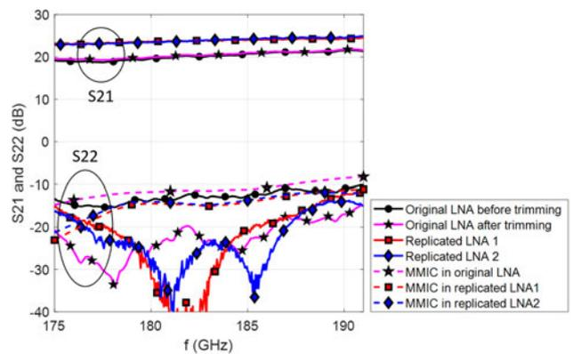
**Fig. 7.** Measured S21 and S22 of two LNAs with redesigned WG-MS transitions compared with original untrimmed measurements and laser trimmed measurements on original module. Measured S22 of MMICs inside original and replicated LNAs are also shown.
