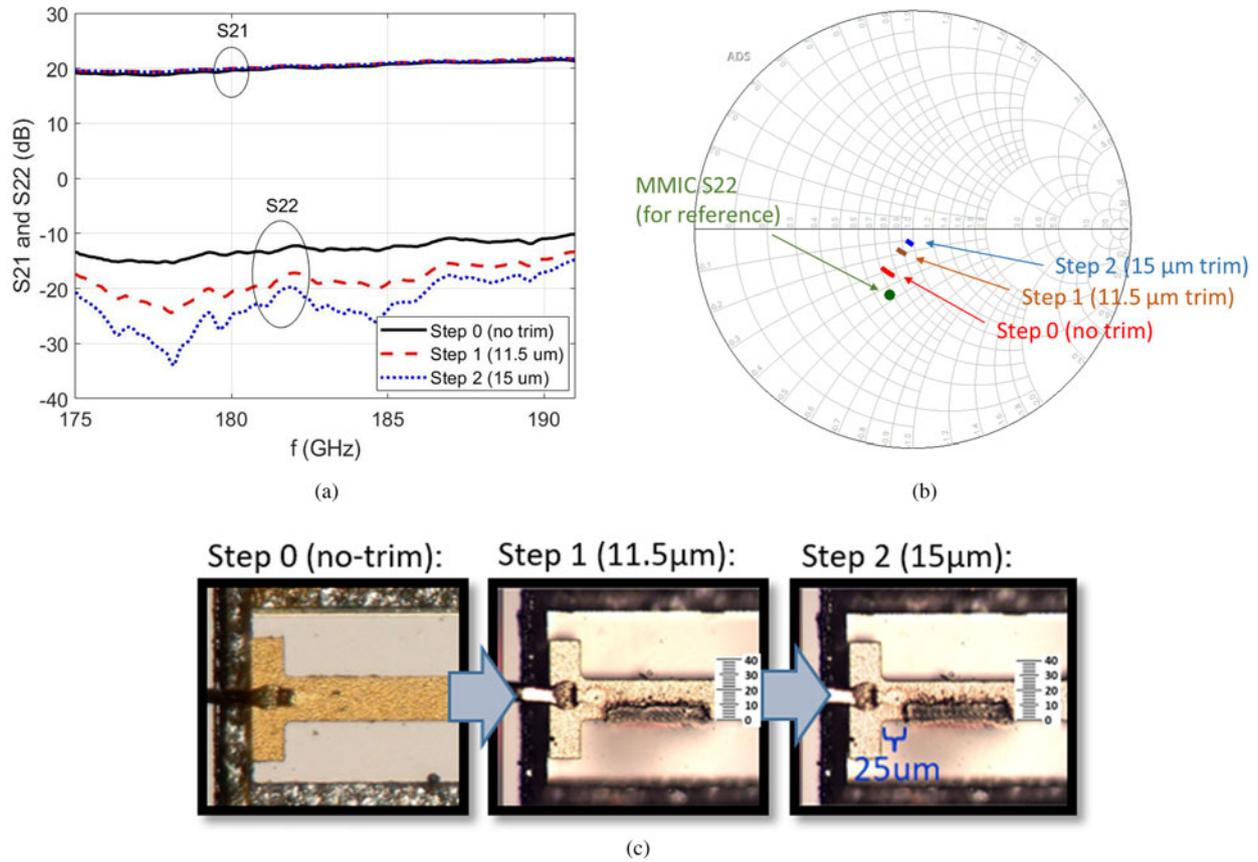
**Fig. 4.** Trimming process on original LNA. (a) Measured S21 and S22 during each trimming step, in Cartesian format. (b) Measured S22 during each trimming step and S22 of the MMIC chip, from 183.2 to 183.4 GHz, on the Smith chart. (c) Microscopic photographs of performed trimming steps.
