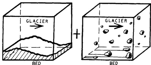
Fig.1. Schematic representation of the basal drag arising from both bed irregularities and rock fragments embedded in the ice. Unlike previous models of sliding, the drag does not necessarily vanish for perfectly smooth beds.
