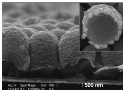
Figure 1. Scanning electron micrograph shows a cross-sectional view of the macroporous  $\text{CaCu}_3\text{Ti}_4\text{O}_{12}$  (CCTO) film formed following calcination at  $800^\circ\text{C}$ . The inset shows one hollow CCTO hemisphere. (Courtesy of Avner Rothschild, MIT.)
