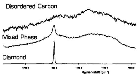
The Raman Microprobe MOLE® can tell you what phase[s] of carbon is present in a matter of seconds:
