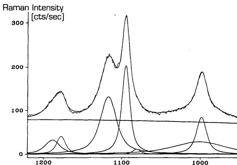
Band Fit of Raman spectrum of glycol group in Polyethylene Terephthalate.
