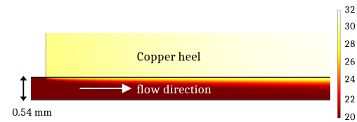
Figure 1: Example of thermal layer within a Poiseuille flow, as computed numerically in section 5.2, in the experimental conditions of Figure 12(a), and a flow velocity of 0.3 m/s. The flow direction is from left to right. The color indicates the copper and water temperature distribution, in Celsius. Thin black lines delineate the copper and water frontiers.
