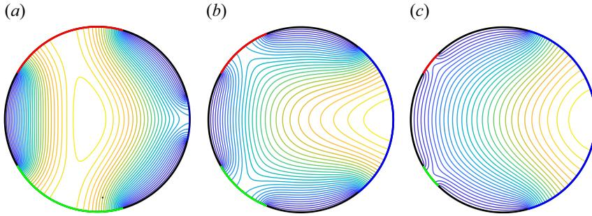
Figure 7. Axial velocity field contour lines for SHS pipes with  $M = 3$  unequal shear-free menisci at  $|z| = 1$  with  $\phi = 1/2$ : (a)  $\Phi = 2.4$ , (b)  $\Phi = 0.9$ , (c)  $\Phi = 1.3$ . The parameters  $r, q, \delta$  are found by solving the three equations in (6.4).
