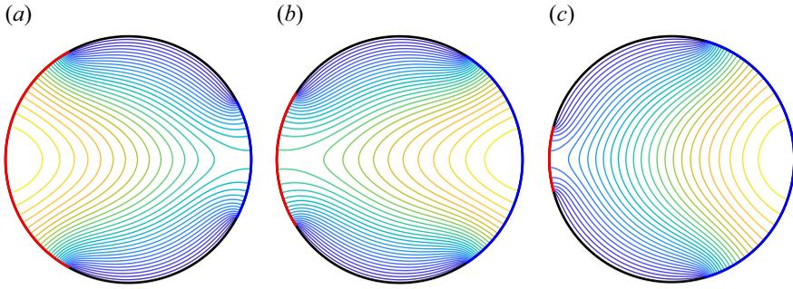
Figure 4. Constant axial velocity contours for superhydrophobic pipes with  $M = 2$  unequal shear-free menisci, assuming  $\phi = 1/2$ : (a)  $\Phi = 1/2$ , (b)  $\Phi = 1$ , (c)  $\Phi = 1.3$ . The parameters  $r, \rho$  are found by solving (5.10).
