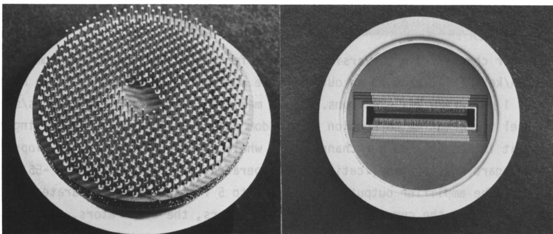
Fig.4 Ceramic header: backside and frontside with mounted array
