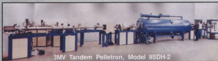
3MV Tandem Pelletron, Model 9SDH-2
