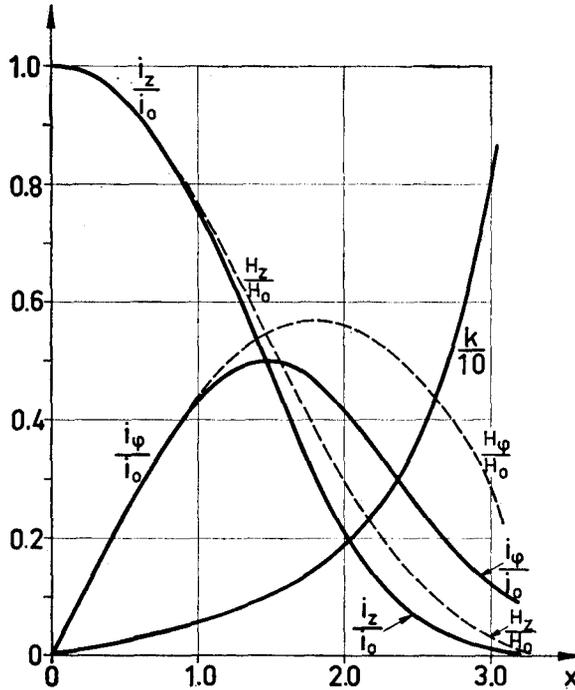
FIG. 2. Axial and azimuthal components of the magnetic field,  $H_z$ ,  $H_\phi$ , of the currents,  $i_z$ ,  $i_\phi$ , and the ratio  $k = H_\phi/H_z$  as functions of the normalized radius  $x = r/b$ .
