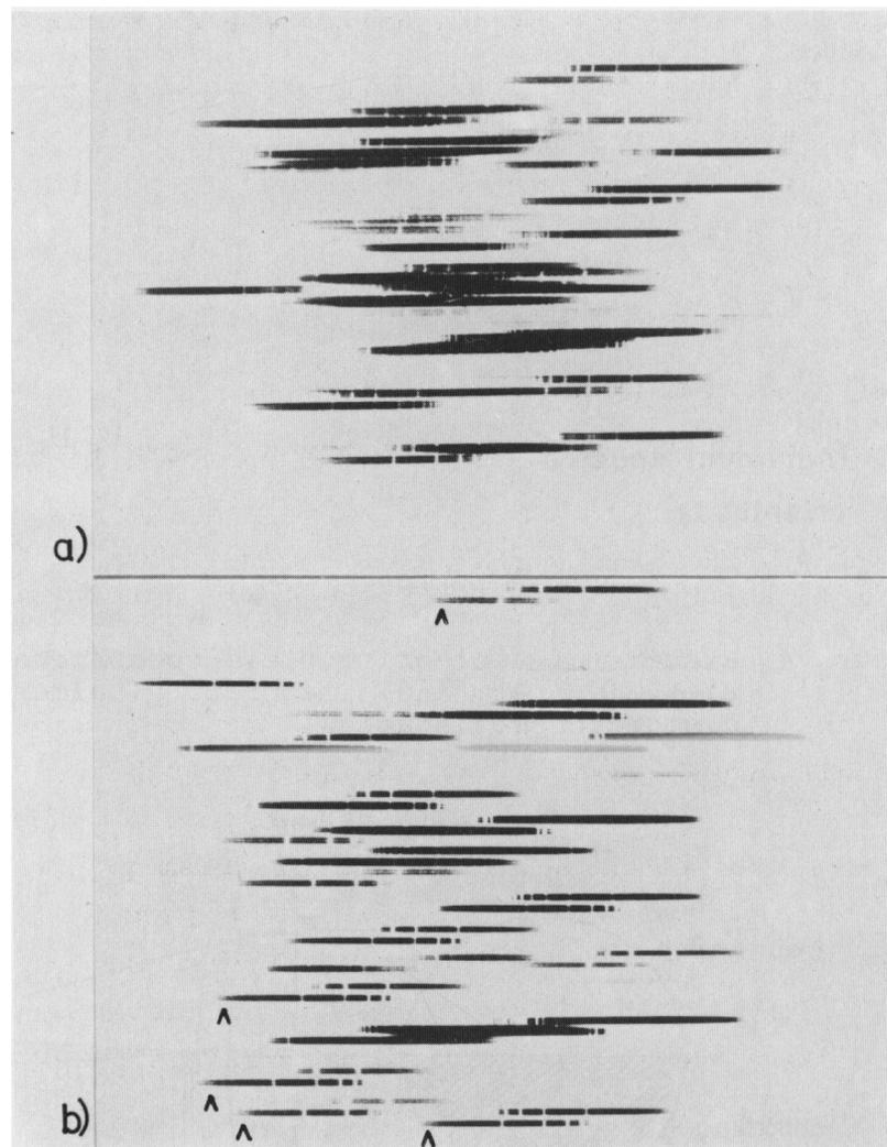
Figure 3: Field spectrogram of NGC 2287 without (a) and with focal plane diaphragm. A double grating prism with 400 grooves/mm was used (217 Å/mm with a  $f=100\text{mm}$  camera). The spectra of fainter objects not visible in the unmasked exposure are marked by arrowheads.
