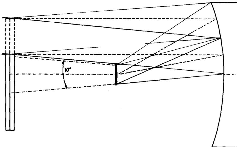
Figure 7: Basic principle of an out of axis Schmidt camera.
