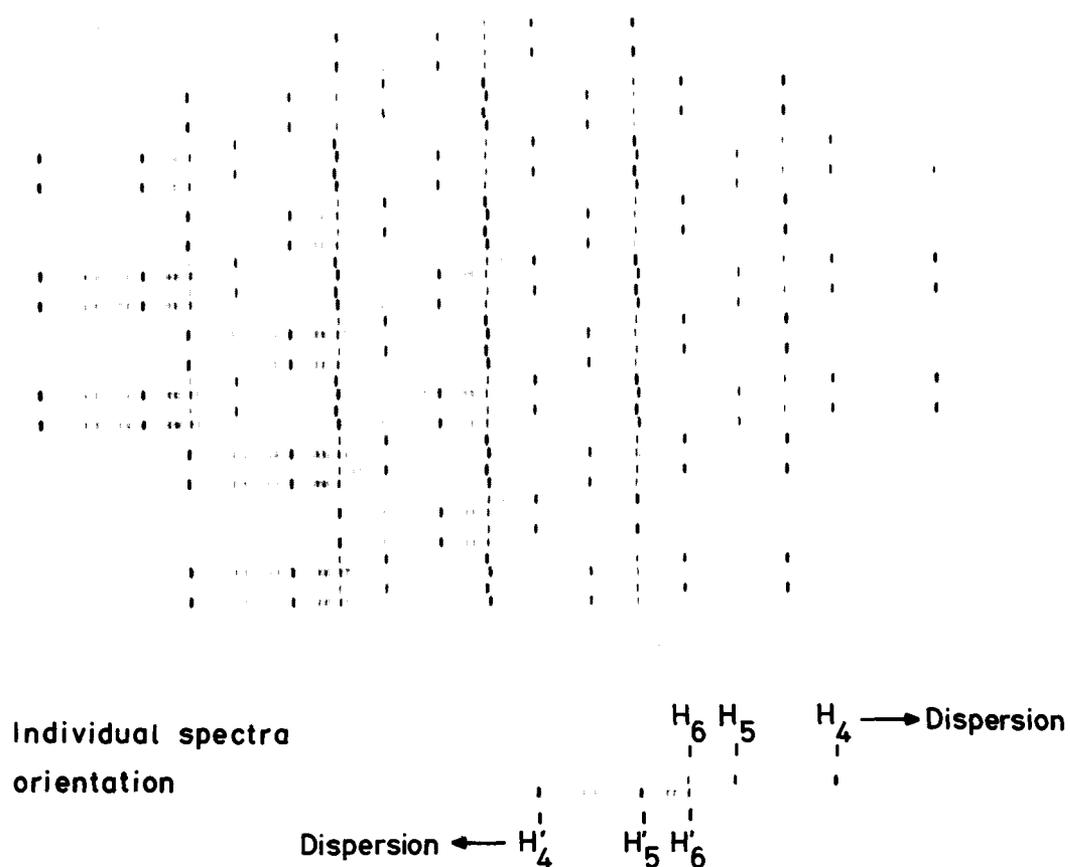
Figure 4: Example of a bi-grism field spectrogram with the multiple slit diaphragm and a laboratory Balmer lamp for field distortion calibration.
