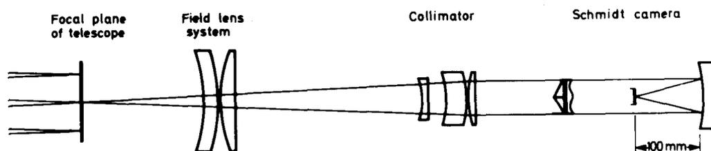
Figure 1: Optical arrangement of the focal reducer of the Hoher List Observatory
