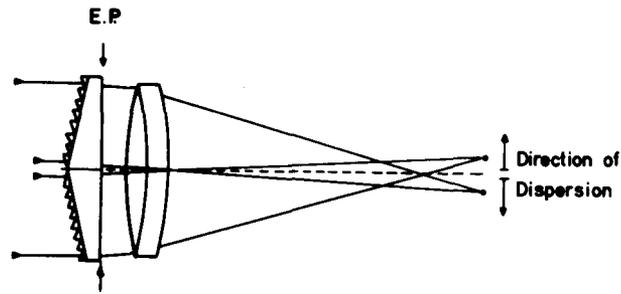
Figure 2: Bi-grism principle for absolute radial velocity determinations with slitless field spectrographs.
