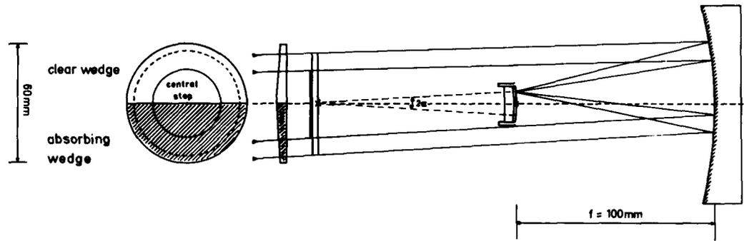
Figure 6: Vignetting free bi-prism Schmidt camera arrangement.
