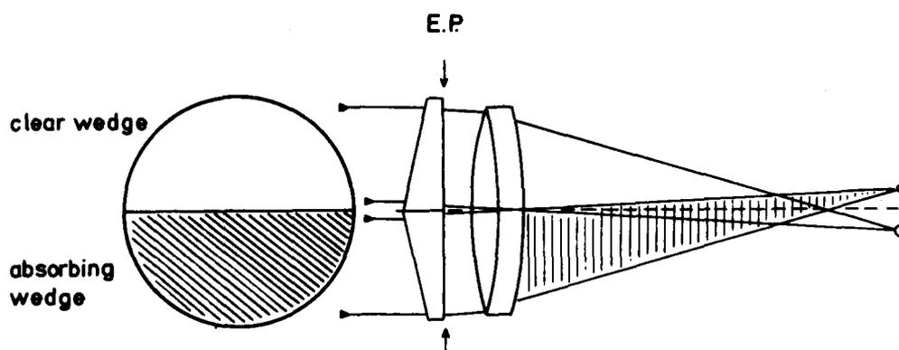
Figure 5: Double wedge principle for autocalibration of panoramic detectors in a focal reducer arrangement.
