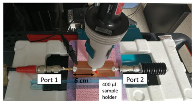
Fig. 4. Detail of the exposure bench during the experimental characterization performed in the presence of a 400 μl sample holder placed at the center of the GCPW line.
