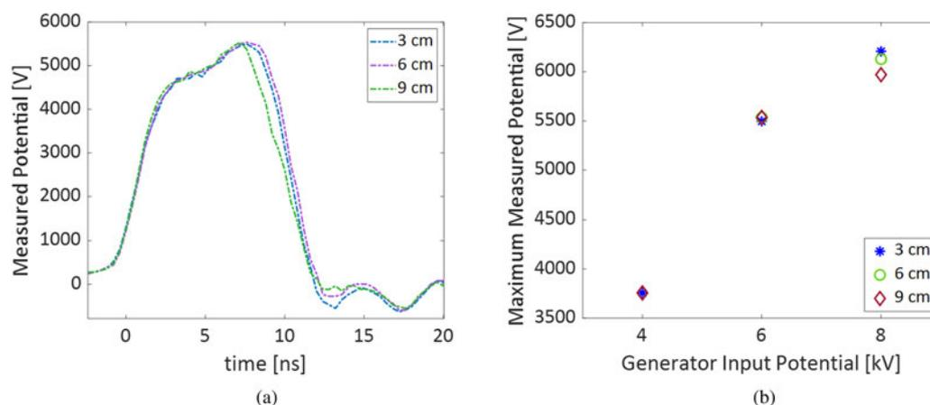
**Fig. 8.** (a) Nanosecond pulse signal measured in time along the exposure system line, at 3, 6, and 9 cm from port 1, setting the generator at 6 kV. (b) Peak values detected measuring the signal along the exposure system line and setting the input potential from the generator at 4, 6, and 8 kV.
