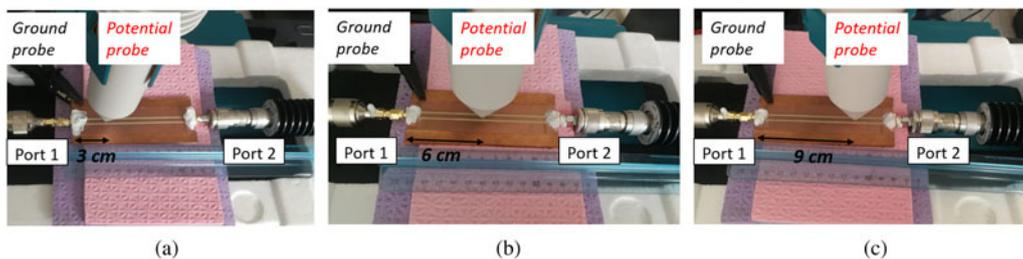
Fig. 3. Detail of the exposure bench during the experimental characterization along the GCPW line, at 3 cm (a), at 6 cm (b), and at 9 cm (c) from port 1.
