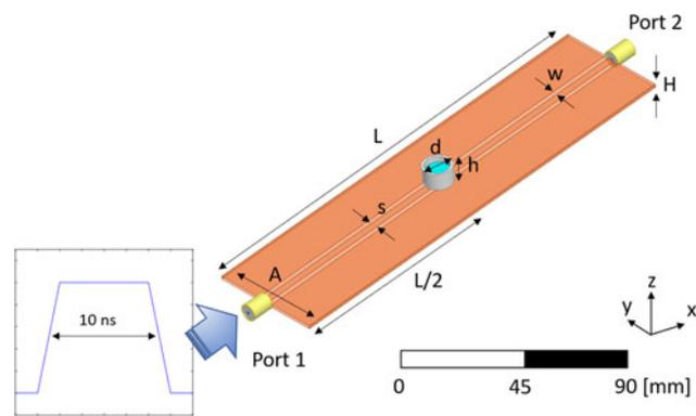
**Fig. 1.** Geometric model of the GCPW structure used for numerical characterization applying a 10 ns duration pulse.
