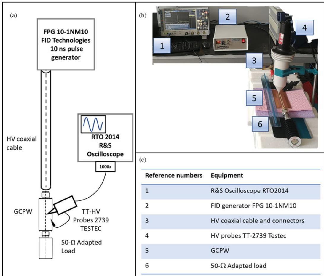
Fig. 2. (a) Scheme of the experimental bench. (b) Experimental bench setup in place. (c) Table of the equipment composing the exposure bench and shown in (b).
