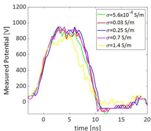
**Fig. 9.** Signals measured inside the five sample solutions with conductivities from  $5.6 \times 10^{-4}$  to 1.4 S/m and the input voltage of 6 kV.
