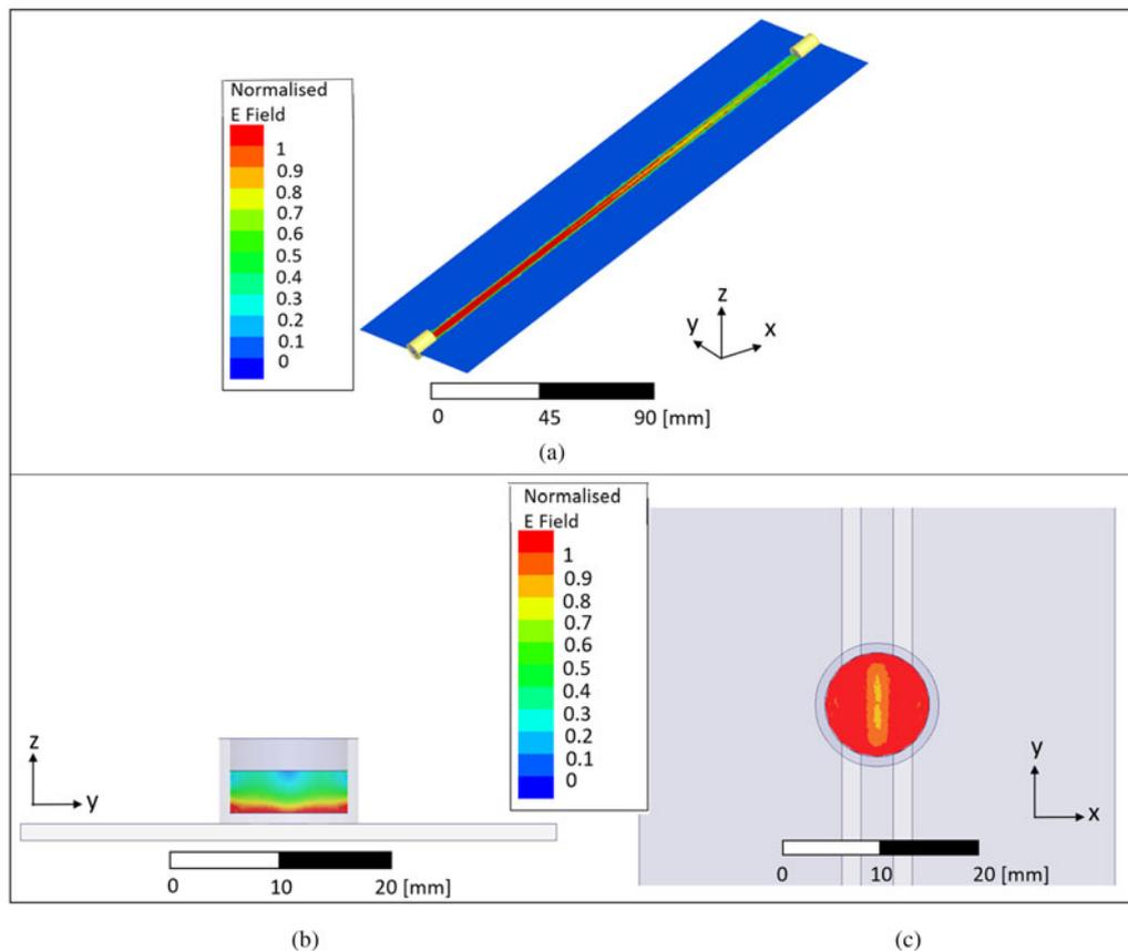
**Fig. 6.** Results of the numerical simulations. (a) Top view of the GCPW with the  $E$  field distribution. (b) Side view of the GCPW with the  $E$  field distribution on the central section of the solution sample. (c) Top view of the GCPW with the  $E$  field distribution at the bottom of the sample holder.
