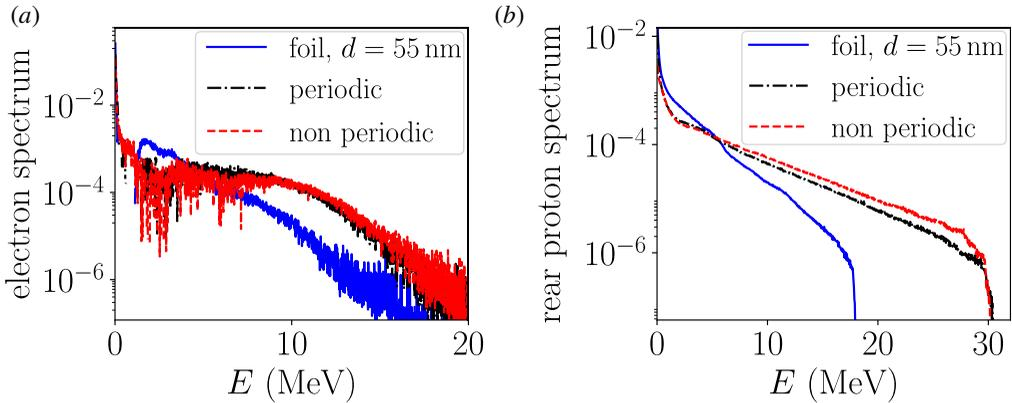
FIGURE 3. Energy spectra of the electrons (a) and rear-protons (b) from a flat foil (solid blue), a  $d = 100$  nm periodic nanohole target (dashed-dotted black) and a  $d = 100$  nm non-periodic nanohole target (dashed red). In (a), only electrons located in the vacuum behind the target backside are considered. Electron spectra are recorded at  $t = 175$  fs and proton spectra at  $t = 455$  fs.
