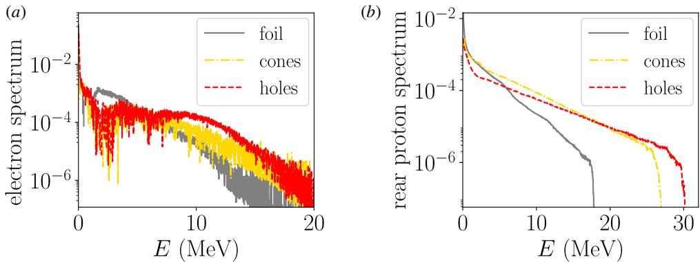
FIGURE 2. Energy spectra of electrons (a) and rear-side protons (b) from a flat foil (solid black), a nanocone (dashed-dotted yellow) and a nanohole (dashed red) target of  $d = 100$  nm thickness. In (a), only electrons located in the vacuum behind the target backside are considered. Electron spectra are recorded at  $t = 175$  fs and proton spectra at  $t = 455$  fs.
