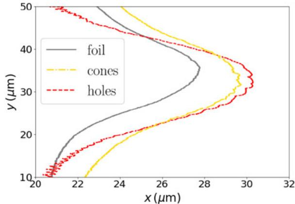
FIGURE 6. Position of the front of the accelerating rear-proton layer at  $t = 175$  fs for a flat foil (solid black), a nanocone (dashed-dotted yellow) and a nanohole (dashed red) targets of  $d = 100$  nm thickness.
