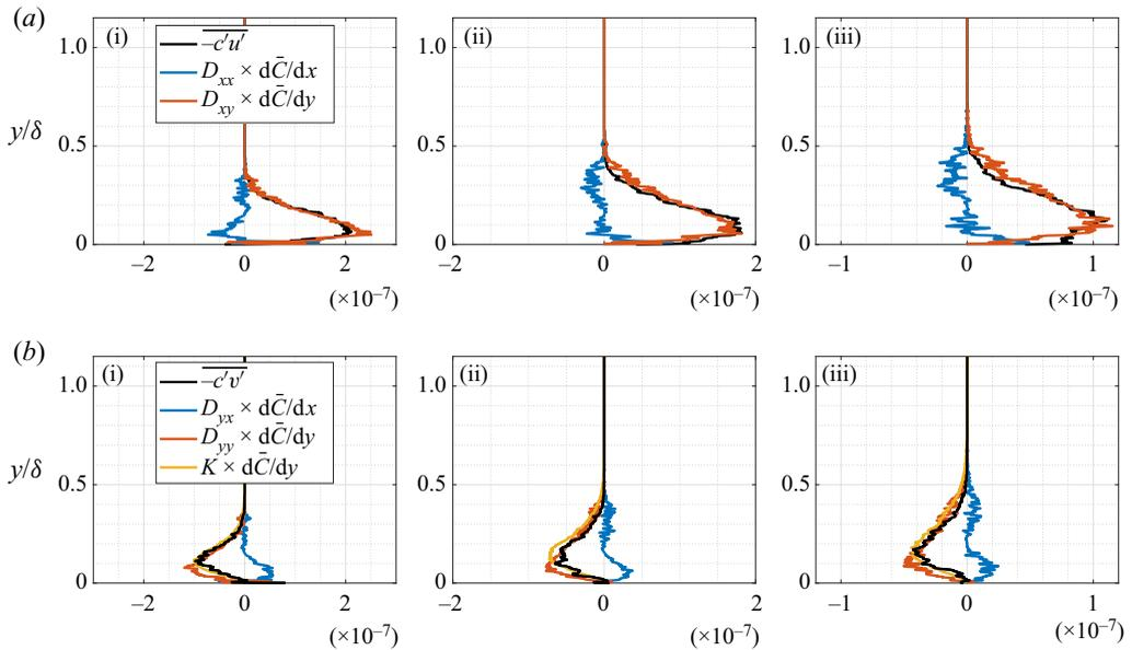
Figure 17. (a,b) Contributions of the concentration gradients to the turbulent scalar fluxes at streamwise locations (i)  $x/\delta = 3.0$ , (ii)  $x/\delta = 4.0$  and (iii)  $x/\delta = 5.0$ . Here  $D_{ij}$  and  $K$  are streamwise-median over  $\pm 0.5x/\delta$  to reduce noise; turbulent fluxes and analytical concentration gradients are extracted at specified locations.
