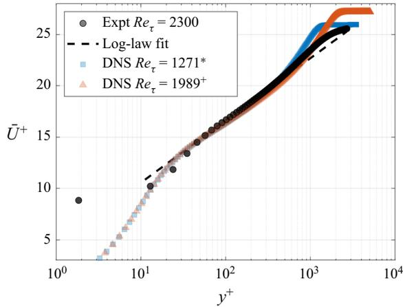
Figure 3. Mean streamwise-averaged velocity profile in inner units with log-law fit based on  $U_\tau = 0.021 \text{ m s}^{-1}$ ,  $\kappa = 0.38$  and  $B = 4.5$ . The DNS data are from \* Schlatter & Örlü (2010) and + Sillero, Jiménez & Moser (2013).
