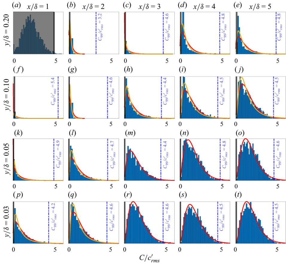
Figure 11. Histograms of  $C/c'_{rms}$  at various wall-normal and streamwise locations. Red lines represent gamma and yellow lines represent lognormal fits. Data within four times the average background noise level in the free stream are shaded grey (note that plot (a) is outside of the plume where no significant concentration is measured).
