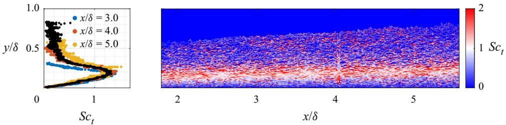
Figure 19. Streamwise-median profile (black) and the corresponding map of the turbulent Schmidt number calculated using the turbulent viscosity and  $D_{yy}$ . Profiles extracted at specified streamwise locations (coloured) are streamwise-median over  $\pm 0.5x/\delta$  to reduce noise.
