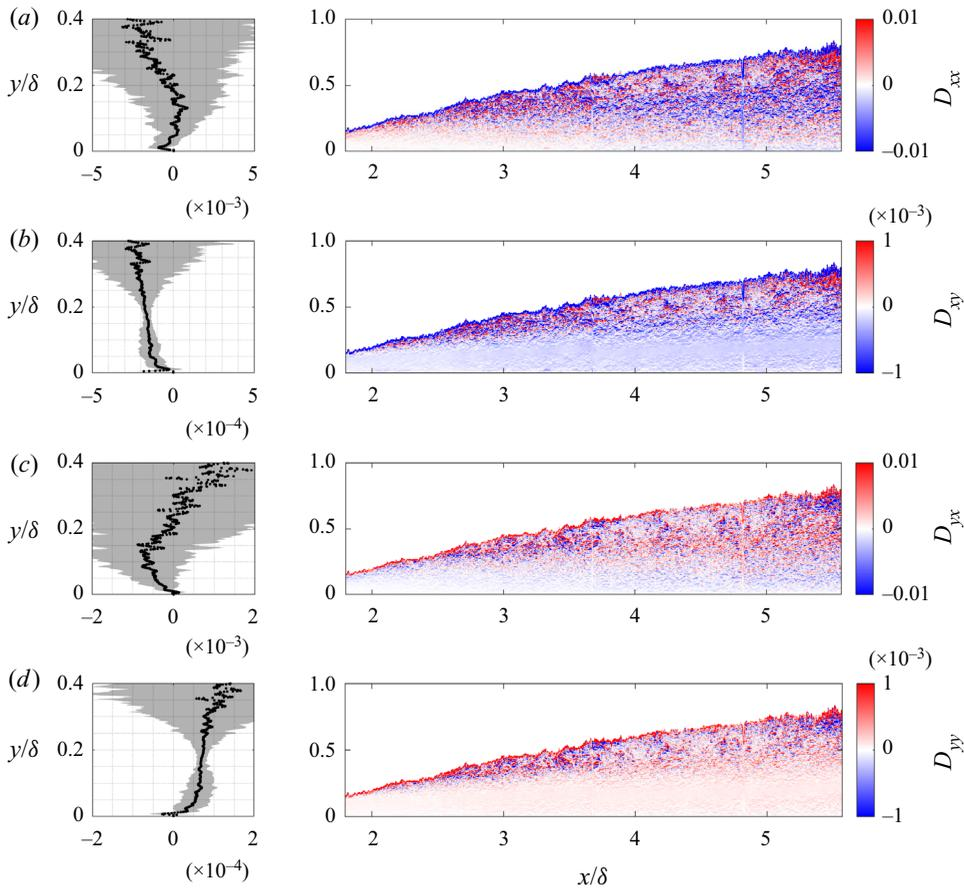
Figure 16. Streamwise-median ( $2.7 < x/\delta < 5.57$ ) profiles and maps of the turbulent diffusivity components: (a)  $D_{xx}$ , (b)  $D_{xy}$ , (c)  $D_{yx}$  and (d)  $D_{yy}$ . The (shading) bounds of the profiles represent one standard deviation of the streamwise variations of the map. Values above  $4.8 \delta_{y,\bar{c}}$  are discarded in the maps.
