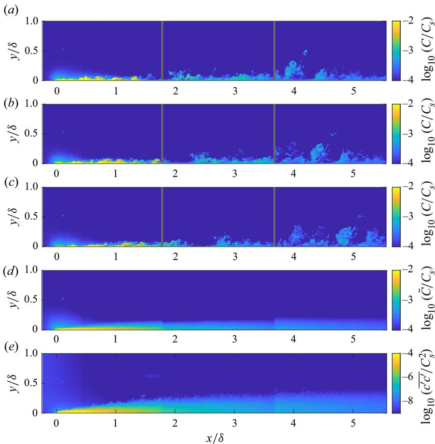
Figure 4. (a–c) Instantaneous concentration fields extracted at  $t/(U_\infty/\delta) = 0.02$  apart with vortical structures trackable across different time frames. Note that each panel is a composite of uncorrelated measurements at P1, P2 and P3, the boundaries of which are denoted by grey lines. (d) Mean concentration and (e) variance fields.
