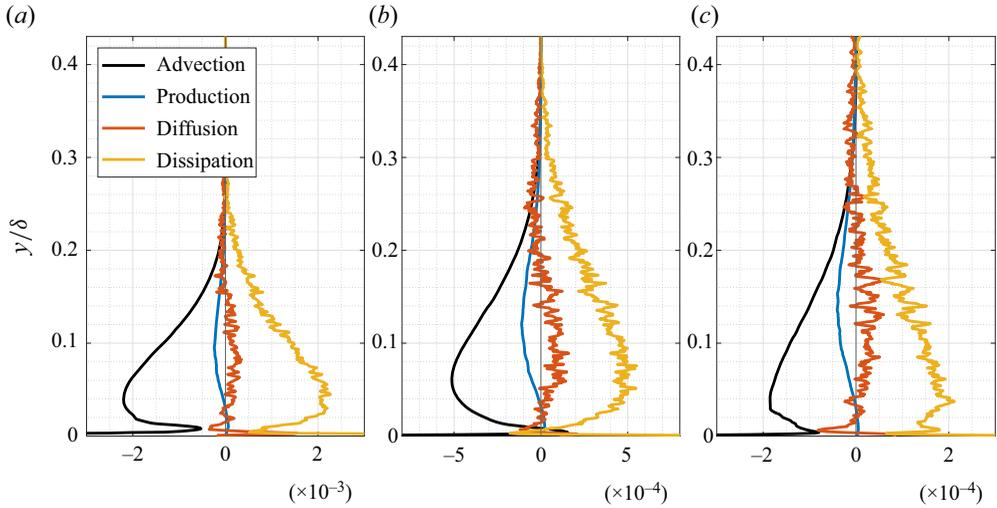
Figure 9. Concentration fluctuations budget at selected streamwise locations: (a)  $x/\delta = 3.0$ , (b)  $x/\delta = 4.0$  and (c)  $x/\delta = 5.0$ . All values are streamwise-median up to  $\pm 0.5x/\delta$  to reduce noise.
