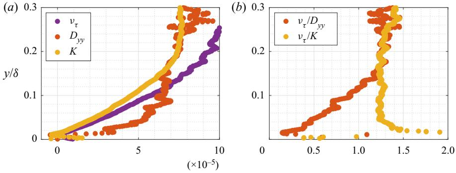
Figure 18. (a) Comparison of the streamwise-median ( $2.7 < x/\delta < 5.57$ ) turbulent viscosity  $v_\tau$  with the turbulent diffusivity obtained using two methods: as  $D_{yy}$ , the dominant component of the turbulent diffusivity tensor, and as  $K$ , the effective turbulent diffusivity coefficient. (b) The streamwise-median ( $2.7 < x/\delta < 5.57$ ) turbulent Schmidt number, i.e. the ratio of the turbulent viscosity and the turbulent diffusivity, based on  $D_{yy}$  and on  $K$ .
