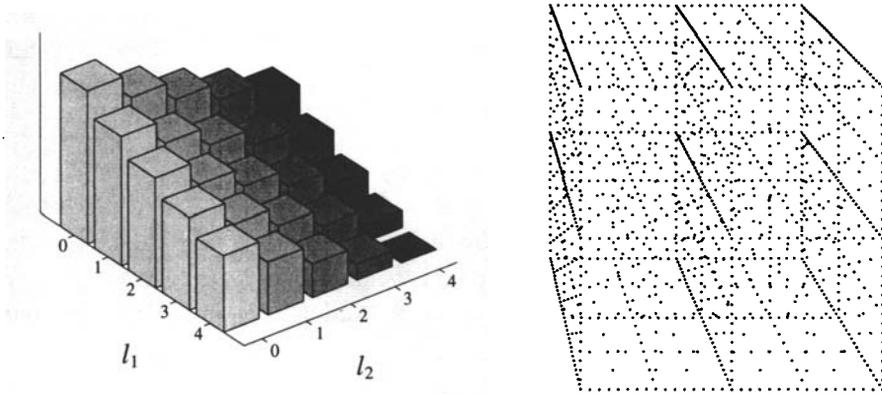
FIGURE 1. Left: Norms of errors of the difference spaces  $W_l$  on a logarithmic scale. The example function is  $u(x_1, x_2) = e^{-(x_1^2+x_2^2)}$  with  $(x_1, x_2) \in [0, 1] \times [0, 1]$ . Right: Sparse grid of refinement level  $l = 5$  in three dimensions.
