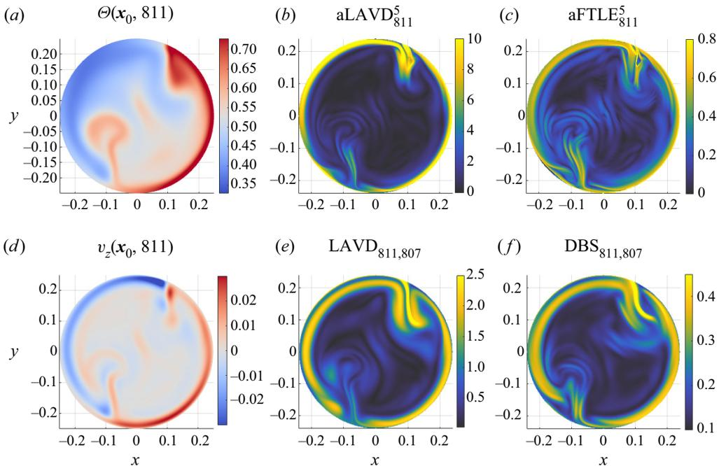
Figure 5. Comparison of temperature and velocity (*a,d*) with active (*b,c*), advective (*e*) and diffusive (*f*) barriers for the rapid rotation case ( $Ro^{-1} = 33$ ) at  $t/t_{ff} = 811$  and  $z/H = 0.1$ . All barrier diagnostics highlight the features of sidewall boundary flow due to convective wall modes.
