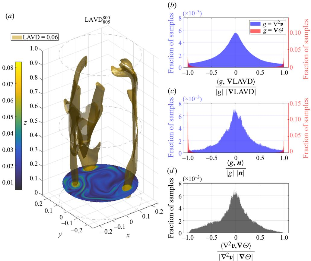
Figure 7. (a) Ekman vortices as LAVD isosurfaces (advective barriers). (b) Inner product of both diffusive heat flux and momentum flux with LAVD gradient. (c) Inner product of both diffusive heat flux and momentum flux with LAVD isosurface normal vectors. (d) Inner product of diffusive heat flux and momentum flux vector along isosurface.
