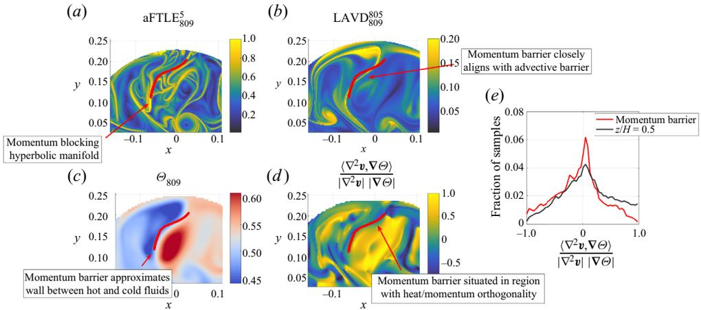
Figure 9. An example hyperbolic manifold in the momentum barrier field intersecting the  $z/H = 0.5$  plane represented as an aFTLE ridge for the  $Ro^{-1} = 0$  flow. This momentum transport barrier is also behaving as a wall between cold and warm regions of the flow, thus maximizing diffusive heat transport.
