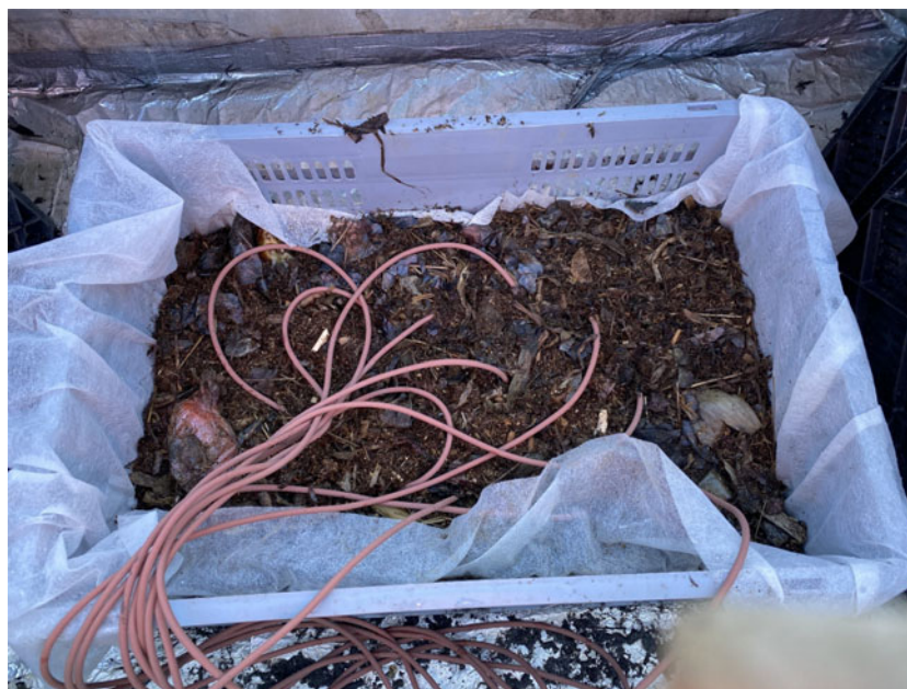
Figure 1. Box with compost consisting of onion waste (60%), horse manure (20%), and wood shavings (20%) and thermocouples mounted at different places in the box.
