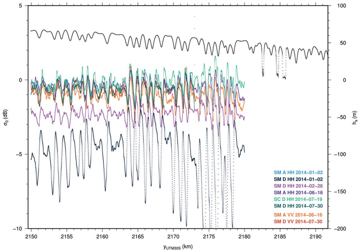
**Fig. 6.** Along-track profile of TerraSAR-X backscatter  $\sigma_0$  in 70 m resolution (bicubic spline interpolation; colours denote date, left vertical axis) and laser scanner data (dark grey, right vertical axis).
