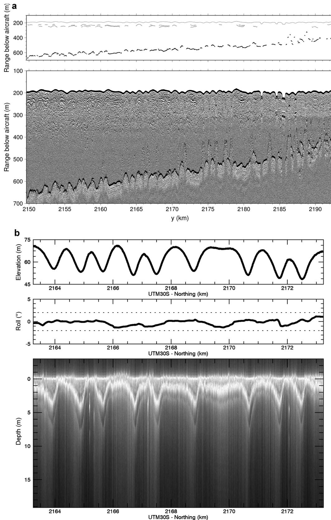
**Fig. 2.** (a) Extracted picks and layering revealed by the RES profile and associated radargram of the ice thickness radar ranging from 200 to 465 m. (b) Subset of the ASIRAS radargram across surface troughs.
