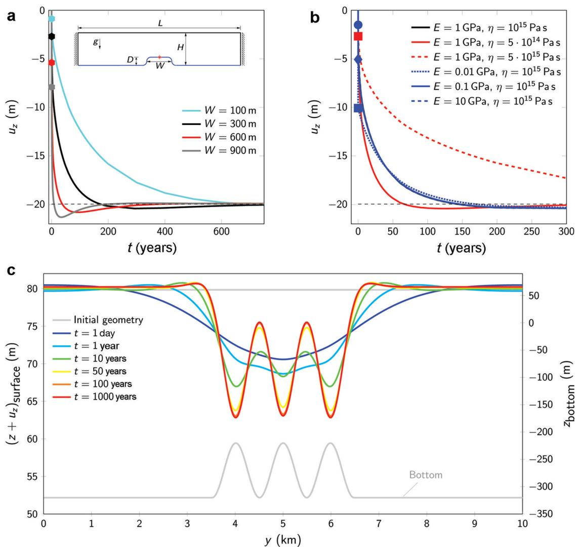
**Fig. 8.** (a) Bottom displacement due to a single crevasse of different width  $W$ . (b) Bottom displacement due to different material parameters  $E$  and  $\eta$  for  $W = 300$  m. (c) Time-dependent surface displacement caused by three crevasses.
