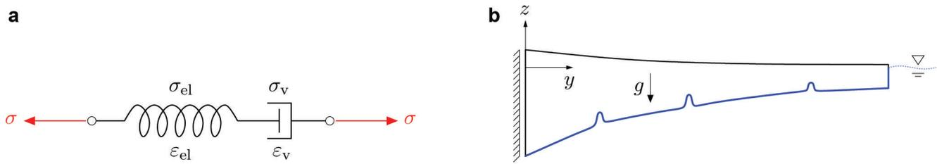
**Fig. 3.** (a) Rheological model of the Maxwell material. (b) Simplified model geometry showing the applied boundary conditions.
