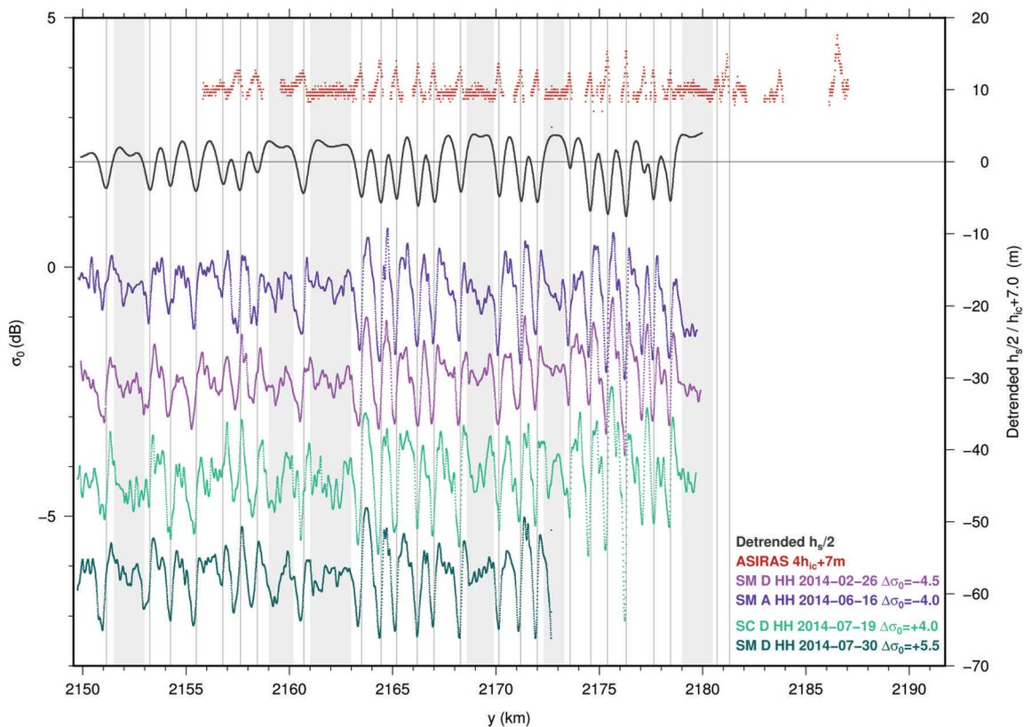
**Fig. 5.** Profile of  $h_{ic}$ , detrended  $h_s$  and  $\sigma_0$  in HH polarization in 70 m resolution (bicubic spline interpolation). The latter are shifted for visibility purposes. Surface troughs are marked as thin vertical lines, undisturbed basal reflection as light grey bars.
