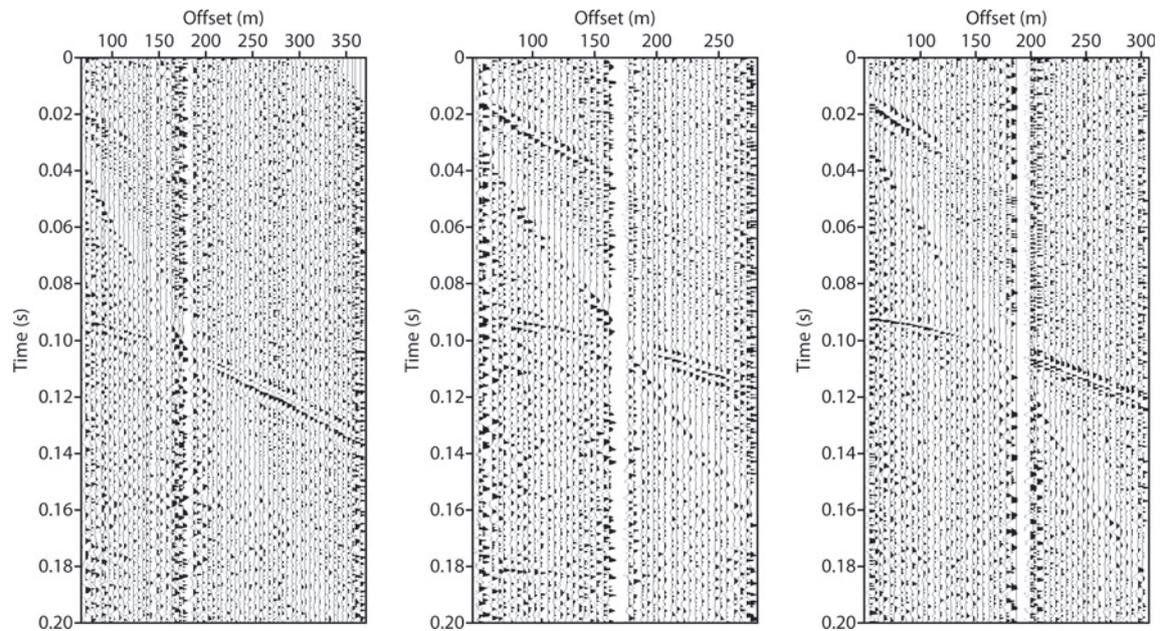
**Fig. 4.** Azimuth-averaged CMP supergathers, from three different locations in the 3-D seismic survey (see Fig. 2 for locations). The bed reflection arrives at  $\sim 90$  ms at near offsets.
