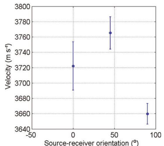
**Fig. 6.** Measured stacking velocities relative to glacier flow. These survey averaged velocities show azimuthal variation of 3.2%. Error bars show the standard deviation over all CMPs for each azimuth. Angles are azimuth relative to flow direction.
