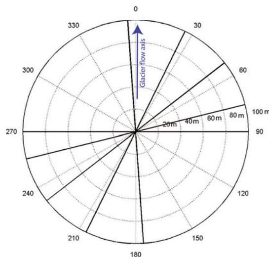
**Fig. 8.** Geometry for the polarimetric GPR CMP gathers as azimuth relative to glacier flow axis. Solid lines show the orientation and length of CMP spreads; maximum offset was 200 m about the common central point.
