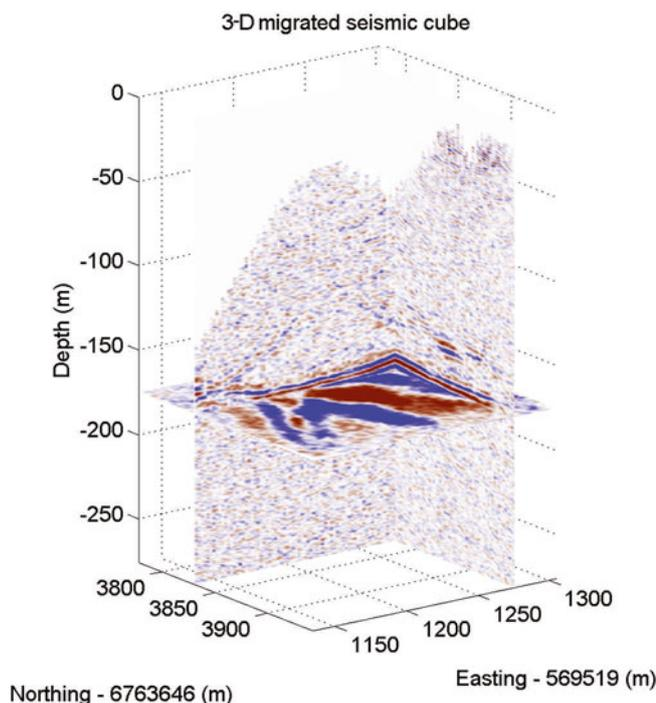
**Fig. 5.** Depth slice through the depth-converted 3-D pre-stack time migrated volume of seismic data showing a detailed image of the bed. Apparent englacial coherent events above the slice depth are migration edge artifacts.
