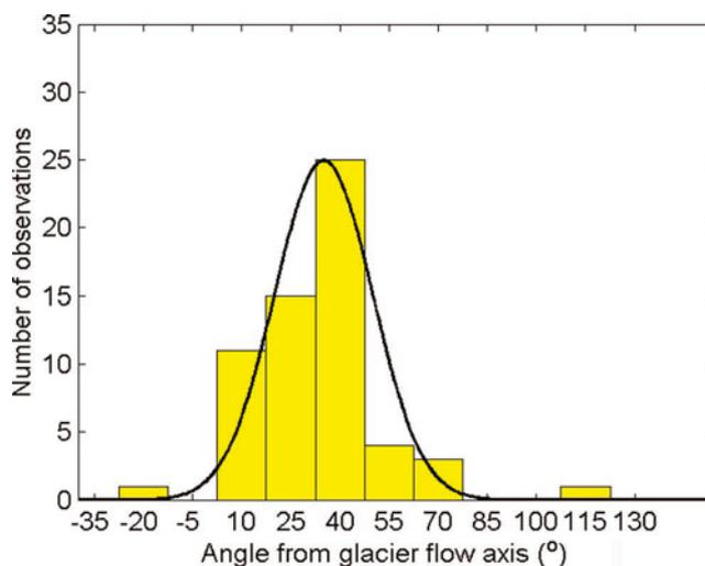
**Fig. 3.** Histogram of vertical fracture azimuth relative to glacier flow axis measured in boreholes on Bench Glacier. While the measured distribution shows some asymmetry, the overlain normal distribution, with standard deviation of  $\pm 15^\circ$ , provides a reasonable description of the variability in crack azimuth.
