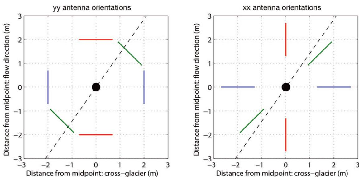
**Fig. 11.** Schematic that illustrates the GPR antenna polarizations at  $0^\circ$ ,  $45^\circ$  and  $90^\circ$  relative to the flow direction for the yy and xx polarizations, along with the estimated fracture direction. In yy polarization, the antennas are never aligned with the fracture direction, so the fast mode is always the first arrival observed from the bed.
