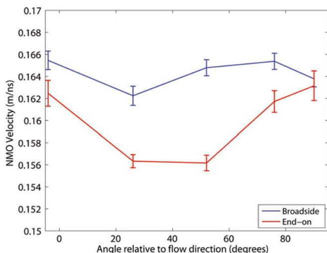
**Fig. 10.** Azimuthal variation in the GPR velocity is distinct and varies with polarization. Error bars show standard deviation in the velocity estimate from NMO analysis. Azimuthal variation is well above the estimated uncertainty of the velocity fit. The slow velocities of  $0.156 \text{ m ns}^{-1}$  between  $26^\circ$  and  $52^\circ$  are measured with the antenna polarization aligned with fracture orientation measured in boreholes and estimated from seismic velocities.
