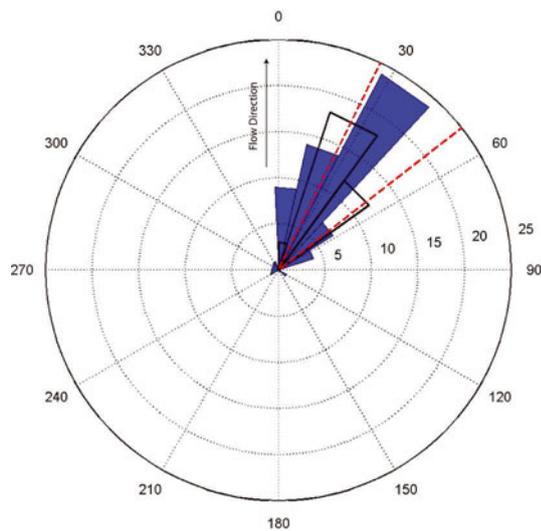
**Fig. 12.** Combined borehole-video (blue), seismic (black outline) and GPR estimates of crack azimuthal distribution (red dash). Angles are relative to the glacier flow direction. All three measurements are consistent and show a preferred orientation of basal crevasses that is oblique to the flow direction at  $\sim 30\text{--}45^\circ$ .
