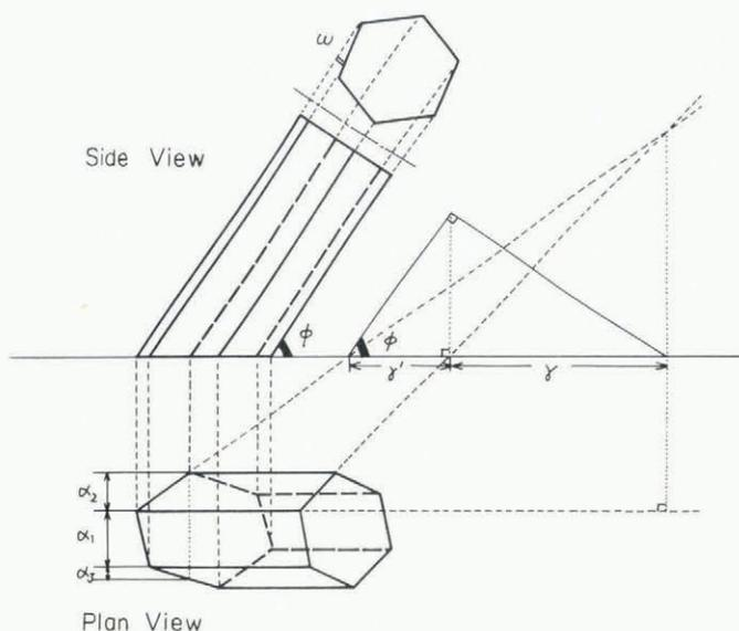
Fig. 2. Geometric configuration of hoar crystal for calculation of crystal orientation.
