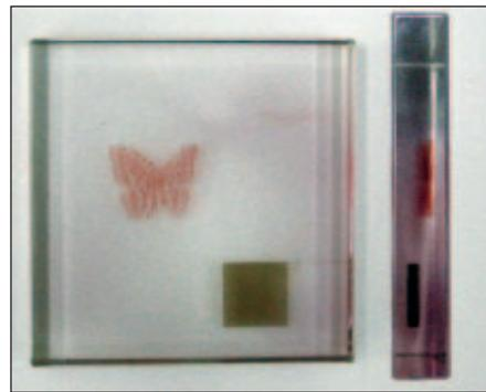
Figure. A butterfly created within a glass sample by femtosecond laser pulse excitation followed by oven annealing. The gray image has not been annealed. The size of the glass sample is 50 mm × 50 mm × 8 mm. The width of the butterfly is ~15 mm. Front and side views are presented.
