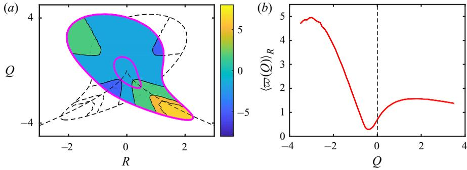
Figure 7. (a) Colour plot of the asymmetry function  $\varpi(Q, R)$ . Isocontours contain 0.7 and 0.85 of the total data. Dashed lines represent the contours of the asymmetry function when  $R \rightarrow -R$ . (b) Asymmetry function averaged along the  $R$  axis,  $\langle \varpi(Q) \rangle_R$ , for  $R$  in the interval  $(-2, 2)$ . Quantities are normalised using  $t_Q = \langle Q^2 \rangle^{1/4}$ .
