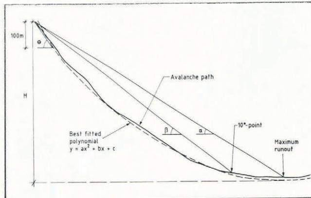
Fig. 3. Terrain parameters used for avalanche run-out calculations.
