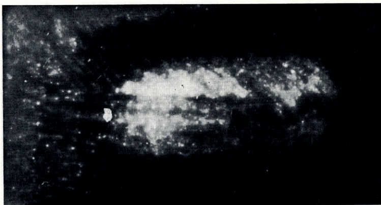
Fig. 3. ^{22}\text{NaCl} segregation in ice crystallized at different velocities; \times 6 .
