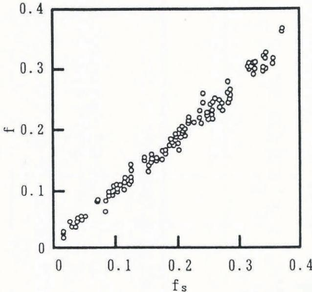
Fig. 7. Indicated fraction,  $f$ , vs sampled fraction,  $f_s$ , by a pipeline system on snow-water mixture.
