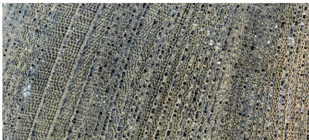
Figure 2 Cross-section scanning image of the experimental archaeological wood (*Zelkova serrata*).
