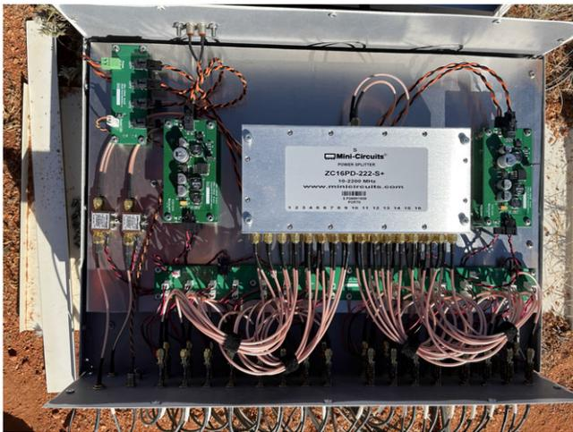
**Figure 6.** The internal architecture of the first-stage beamformer connected to the sixteen dipoles from the southeast section of the CRAM. The first-stage beamformer houses a power combiner, DC-DC converter and additional power supply units to power the boards.
