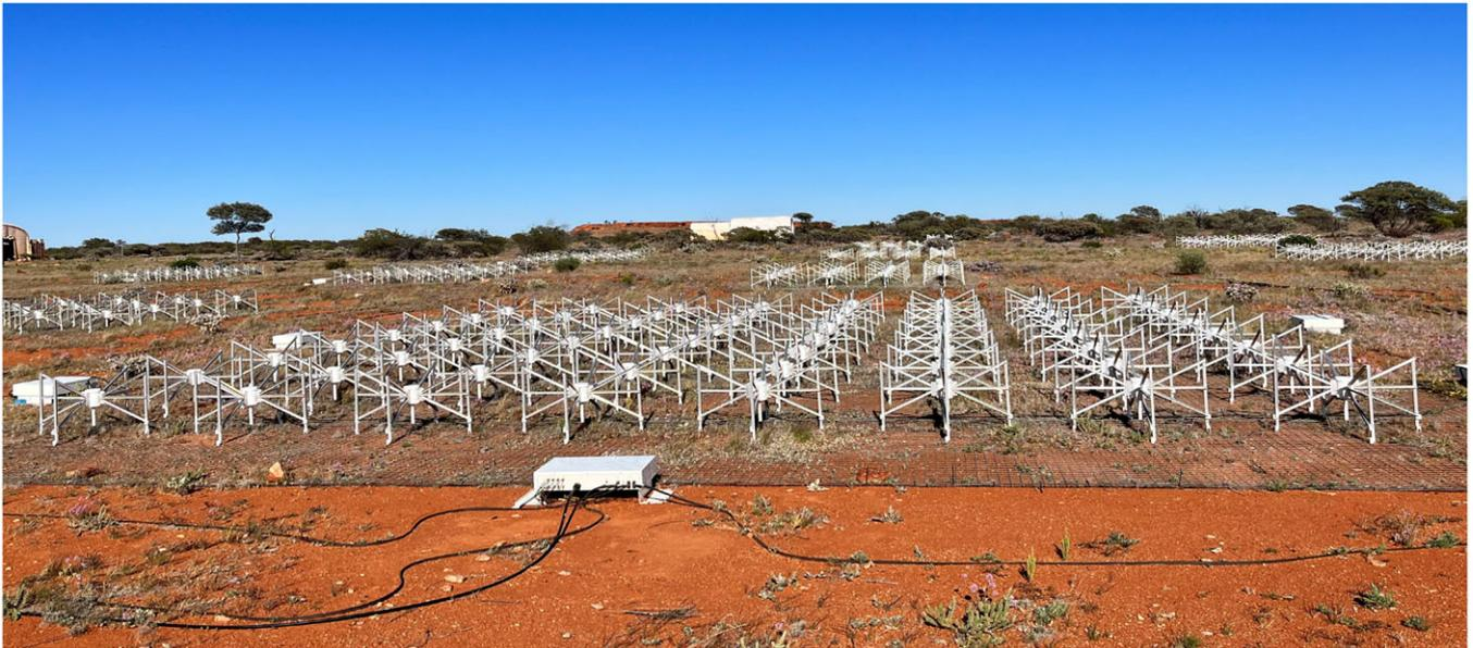
**Figure 3.** The CRAM as installed at the centre of the southern hexagon array of the MWA Phase II configuration, looking west. In the lower centre of the image is the second-stage beamformer, first-stage beamformers are visible on the left and right of the image.
