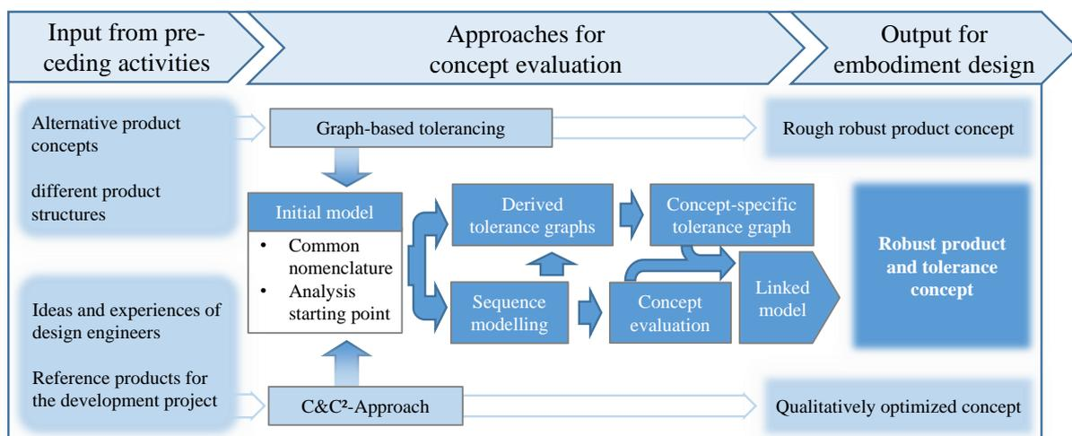
Figure 3. Embodiment-function-driven tolerancing - combination of graph-based tolerancing and C&C<sup>2</sup>-Approach
