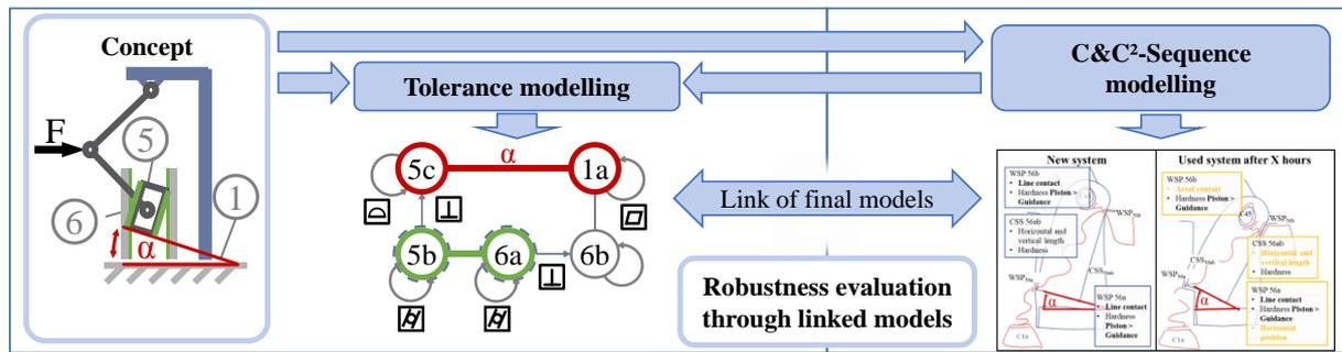
**Figure 8.** Enhanced tolerance structure graph of the relevant loop for the functional key characteristic  $\alpha$  with link to C&C<sup>2</sup>-Model of detailed EFRs
