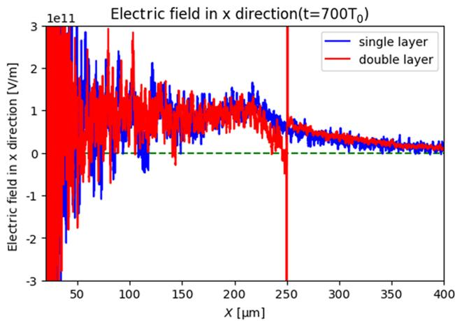
**Figure 10.** Electric field intensity distribution versus position for ps laser-driven single target and double-film target conditions. The data are from Figures 7(b) and 7(d). The blue line is for a single target and the red line is for a double-film target.
