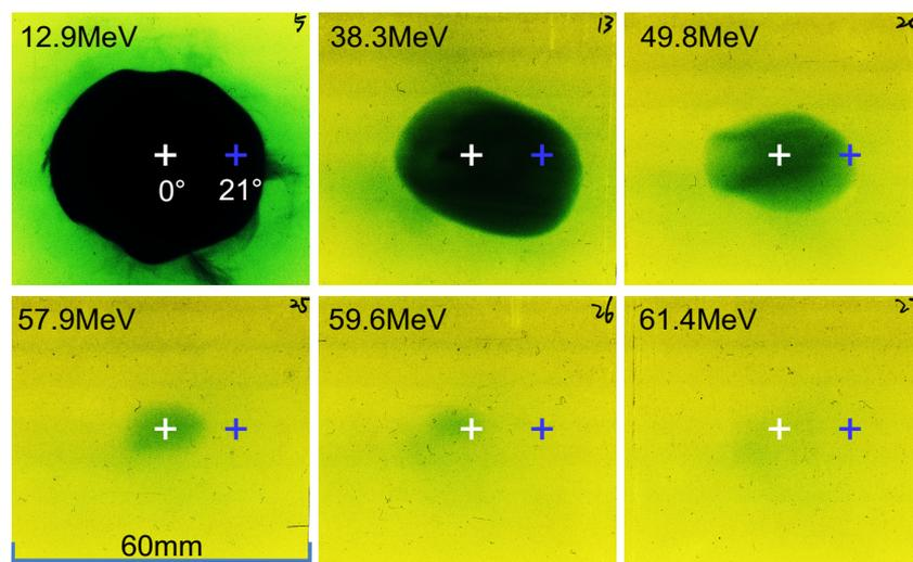
Figure 5. Several images of different layers of radiochromic film (RCF) sheets showing proton signals with different proton energies.
