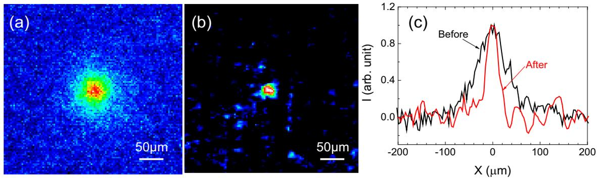
**Figure 3.** X-ray images and scanned intensity curve of the laser irradiating metal planar target: (a) image before optimization; (b) image after optimization; (c) scanned intensity curve along the  $x$ -direction.
