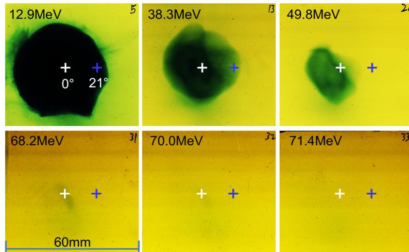
**Figure 8.** Several images of different layers of RCF sheets showing the proton beam output with higher cutoff energy using a double-film target.
