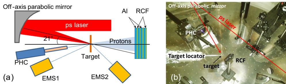
**Figure 4.** Light path and diagnostic arrangement of a laser-driven proton acceleration (LDPA) experiment based on the target normal sheath acceleration (TNSA) mechanism. (a) Schematic of the arrangement. (b) Photograph of the target chamber.
