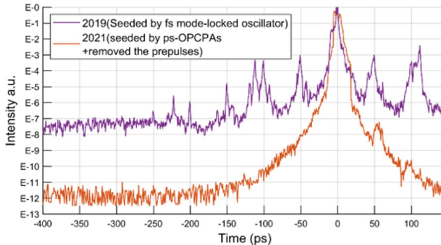
**Figure 2.** Comparison of the signal-to-noise ratio of the front-end optical parametric chirped pulse amplification (OPCPA) output of the picosecond pulse before and after optimization.
