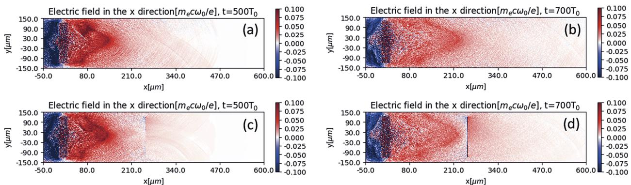
**Figure 7.** Two-dimensional spatial distribution of electric field intensity for ps laser-driven single- and double-film targets. (a), (b) Single target and (c), (d) double-film target; (a), (c) at  $500T_0$  and (b), (d) at  $700T_0$ .
