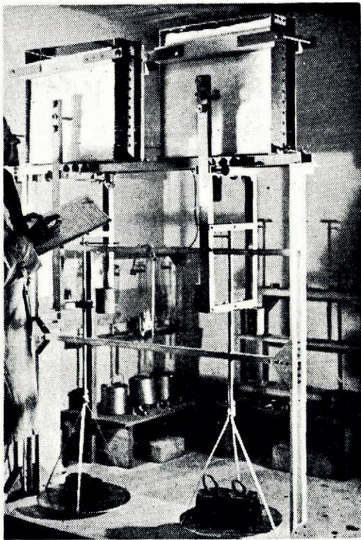
*Apparatus for measuring plasticity of snow*
