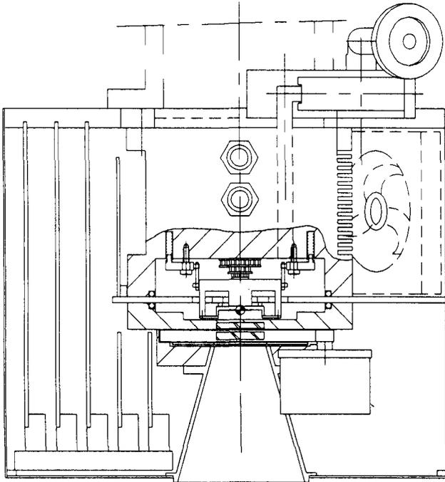
Figure 1. The CCD camera with its shutter and filterwheel and associated electronics is located in a compact housing at the position of the previous plate holder. The camera is thermally neutral as the heat from the electronics and the warm end of the Peltier elements is removed by circulating water.
