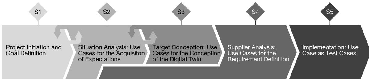
Figure 1. Procedure model for the conception and implementation of a Digital Twin in industry
