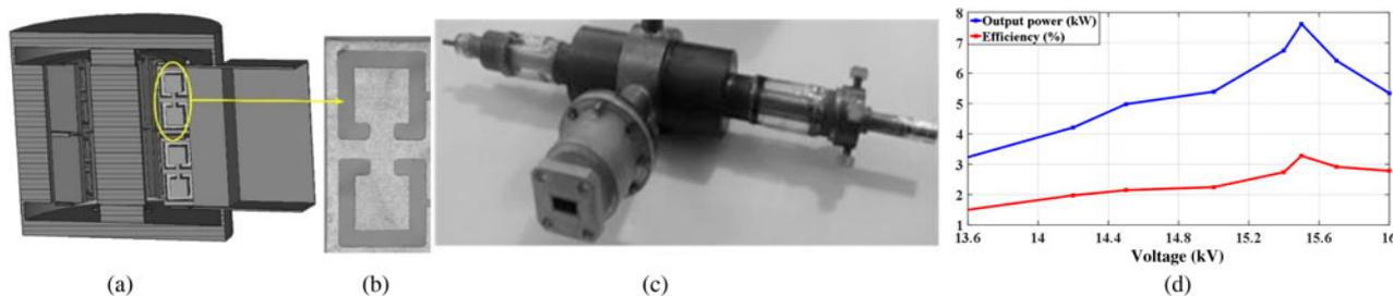
**Fig. 5.** (a) CSOLR-loaded SHM, (b) CSOLRs which have been cut using EDM technique on a side wall, (c) the assembled magnetron, and (d) measured output power and efficiency.
