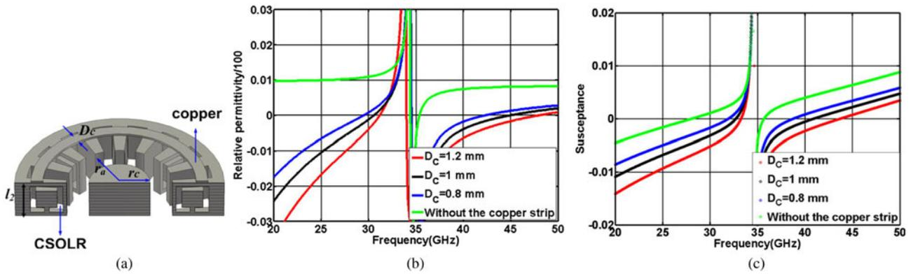
Fig. 3. (a) MCSOLR-loaded SWS. Dimensions of the MCSOLR, unit-cell, and the interaction space are (see Fig. 2(c))  $l_1 = 1.6$  mm,  $l_2 = 1.724$  mm,  $g = 0.2$  mm,  $w = 0.25$  mm,  $D = 1.4$  mm,  $t = 0.39$  mm,  $h_1 = h_2 = 0.49$  mm,  $r_c = 1.3$  mm, and  $r_a = 2.25$  mm; (b) retrieved relative permittivity; and (c) calculated  $B_{int}(\omega) + B_{res}(\omega)$ .
