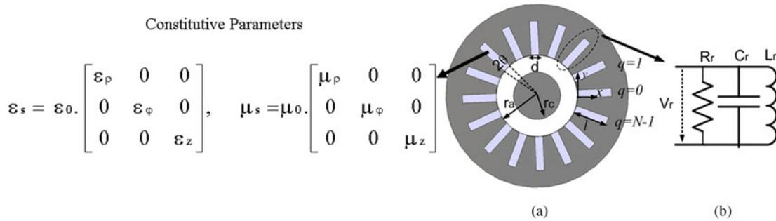
Fig. 1. (a) SWS of a loaded with an anisotropic medium and (b) equivalent circuit of the side resonators.
