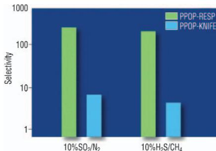
Figure 1. Comparison of the selectivity of poly[bis(phenoxy)phosphazene] (PPOP) membranes prepared by the rapid evaporative spray process (RESP) and by conventional knife-casting.
