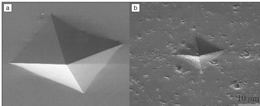
Figure 1. (a) Indentation made in stainless steel by a Vickers indenter; and (b) indentation made with the same indenter and load into  $B_4C$ . The comparatively small indentation mark in  $B_4C$  is an indication of its hardness.
