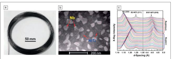
Figure 3. Elastic strain engineering of kilogram-scale Nb nanowires (a-b) is made possible by coupling them to a NiTi shape-memory matrix (b) "loader." Completely reversible change in Nb lattice spacing, up to one million loading-unloading cycles, was demonstrated by in situ synchrotron x-ray diffraction (c). Figure is reprinted with permission from Reference 35. © 2013 AAAS.
