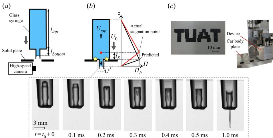
**Figure 1.** (a) The device before the impact. (b) The device just right after the impact. The observation result ( $v = 100 \text{ mm}^2 \text{ s}^{-1}$ ) (bottom) and  $\Pi$ - $z$  diagram (right). (c) Result of using the new on-demand painting system (left) and the entire device (right).
