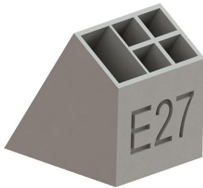
**Figure 2.** Study participants were asked to improve the manufacturability of a pencil holder with an engraved logo while maintaining cosmetic and functional constraints. The pencil holder is shown here with the class number.
