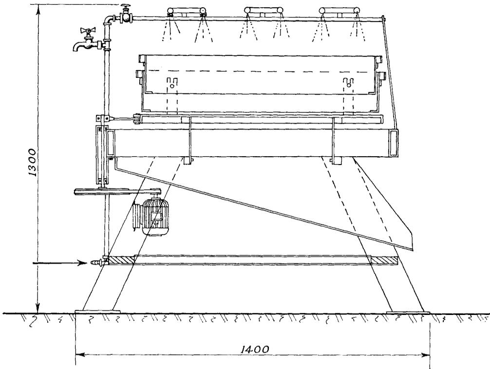
Fig. 1. Technical drawing of the mechanical sieve
