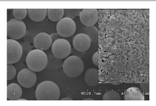
Scanning electron micrograph of calcium phosphate cements-collagen composite microparticle morphology and surface microstructure (inset) prepared by aqueous emulsification at room temperature.
