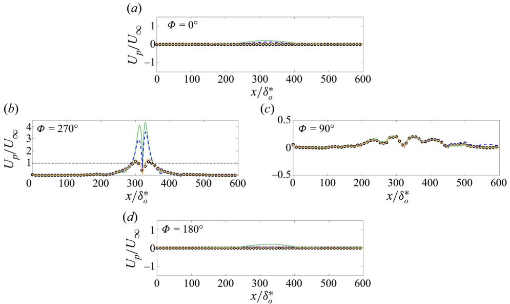
Figure 13. Streamwise distribution  $U_p/U_\infty$ . Only the main four phases of the cycle are shown. Colours are as follows: ● steady case; green solid line,  $k = 10$ ; blue dashed line,  $k = 1$ ; orange dash-dotted line,  $k = 0.2$ .
