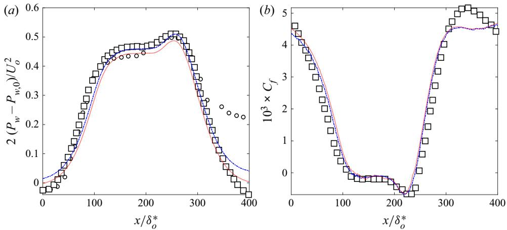
Figure 3. Distribution of (a) the mean pressure coefficient  $C_p$  and (b) the skin-friction coefficient  $C_f$ . Blue dashed line,  $1536 \times 192 \times 256$  mesh; red dashed line,  $1152 \times 129 \times 152$  mesh;  $\square$  Abe (2017);  $\circ$  Weiss *et al.* (2015).
