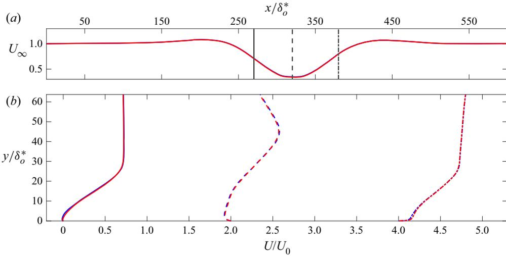
Figure 2. (a) Free-stream velocity  $U_\infty$  (black lines represent the locations where the velocity profiles are extracted), and (b) mean velocity at three different streamwise locations. Blue lines denote the  $1536 \times 192 \times 256$  grid; red lines denote the  $1152 \times 129 \times 152$  grid.
