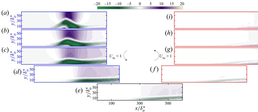
Figure 22. Contours of the percentage difference  $\Delta u$  (3.2) for the case  $k = 0.2$ . Axis colours follow the schematic in figure 17: (a)  $\Phi = 288^\circ, 252^\circ$ ; (b)  $\Phi = 306^\circ, 234^\circ$ ; (c)  $\Phi = 324^\circ, 216^\circ$ ; (d)  $\Phi = 342^\circ, 198^\circ$ ; (e)  $\Phi = 0^\circ, 180^\circ$ ; (f)  $\Phi = 18^\circ, 162^\circ$ ; (g)  $\Phi = 36^\circ, 144^\circ$ ; (h)  $\Phi = 54^\circ, 126^\circ$ ; (i)  $\Phi = 72^\circ, 108^\circ$ .
