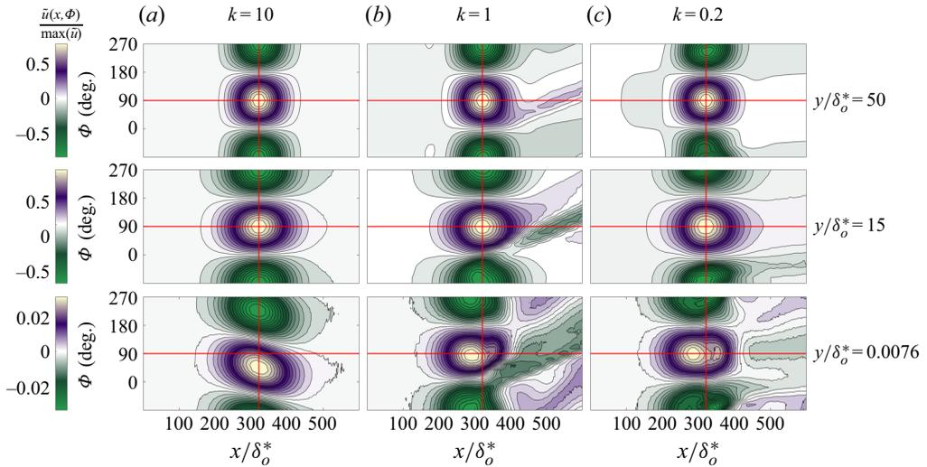
Figure 23. Contours of coherent component  $\tilde{u}$  as a function of the phase angle  $\Phi$  for the three reduced frequencies  $k$  and three wall-normal locations corresponding to: wall ( $y/\delta_o^*=0.0076$ ), outer layer ( $y/\delta_o^*=15$ ) and free stream ( $y/\delta_o^*=50$ ).
