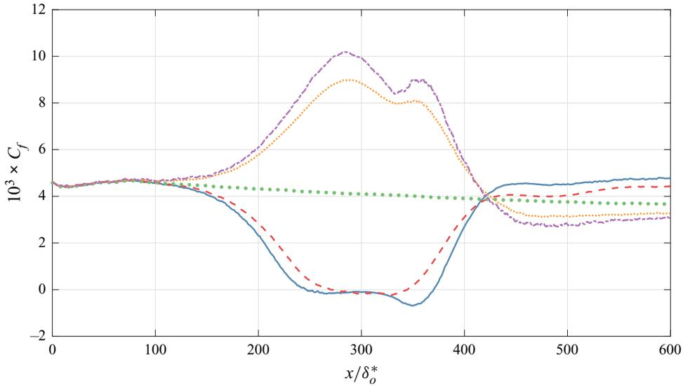
Figure 6. Spatial distribution of the skin-friction coefficient  $C_f$  for the steady calculations corresponding to the following phases: blue solid line, SC-1  $\Phi = 270^\circ$ ; red dashed line, SC-2  $\Phi = 306^\circ$ ; green dotted line, SC-3  $\Phi = 0^\circ$ ; orange dotted line, SC-4  $\Phi = 54^\circ$ ; purple dash-dotted line, SC-5  $\Phi = 90^\circ$ .
