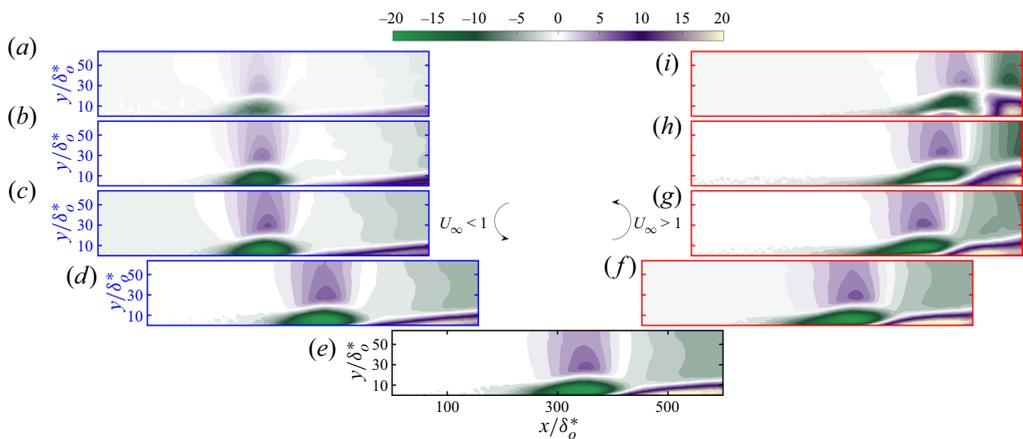
Figure 21. Contours of the percentage difference  $\Delta u$  (3.2) for the case  $k = 1$ . Axis colours follow the schematic in figure 17: (a)  $\Phi = 288^\circ, 252^\circ$ ; (b)  $\Phi = 306^\circ, 234^\circ$ ; (c)  $\Phi = 324^\circ, 216^\circ$ ; (d)  $\Phi = 342^\circ, 198^\circ$ ; (e)  $\Phi = 0^\circ, 180^\circ$ ; (f)  $\Phi = 18^\circ, 162^\circ$ ; (g)  $\Phi = 36^\circ, 144^\circ$ ; (h)  $\Phi = 54^\circ, 126^\circ$ ; (i)  $\Phi = 72^\circ, 108^\circ$ .
