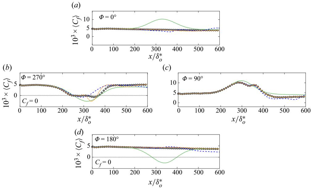
Figure 16. Distribution of phase-averaged skin-friction coefficient ( $C_f$ ) for four phases in the cycle for the different reduced frequencies  $k$ . • Steady case; green solid line,  $k = 10$ ; blue dashed line,  $k = 1$ ; red dash-dotted line,  $k = 0.2$ .
