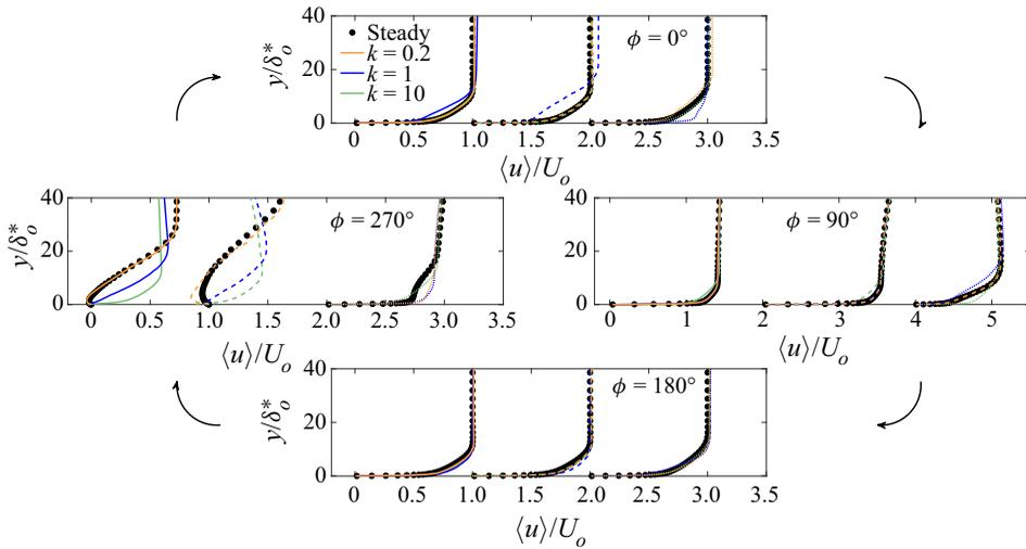
Figure 14. Streamwise phase-averaged  $\langle u \rangle$  velocity profile for four phases in the cycle for the different reduced frequencies  $k$  (colours) and streamwise locations (line styles). Comparison is made with steady calculations (symbols) at the same streamwise locations. Each profile is shifted by one unit for clarity. Solid line,  $x/\delta_o^* = 270$ ; dashed line,  $x/\delta_o^* = 300$ ; dotted line,  $x/\delta_o^* = 450$ .
