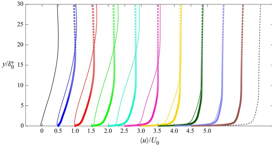
Figure 19. Phase-averaged streamwise velocity for the  $k = 1$  case at the streamwise location  $x/\delta_0^* = 300$ . The same notation as in figure 18 is used.
