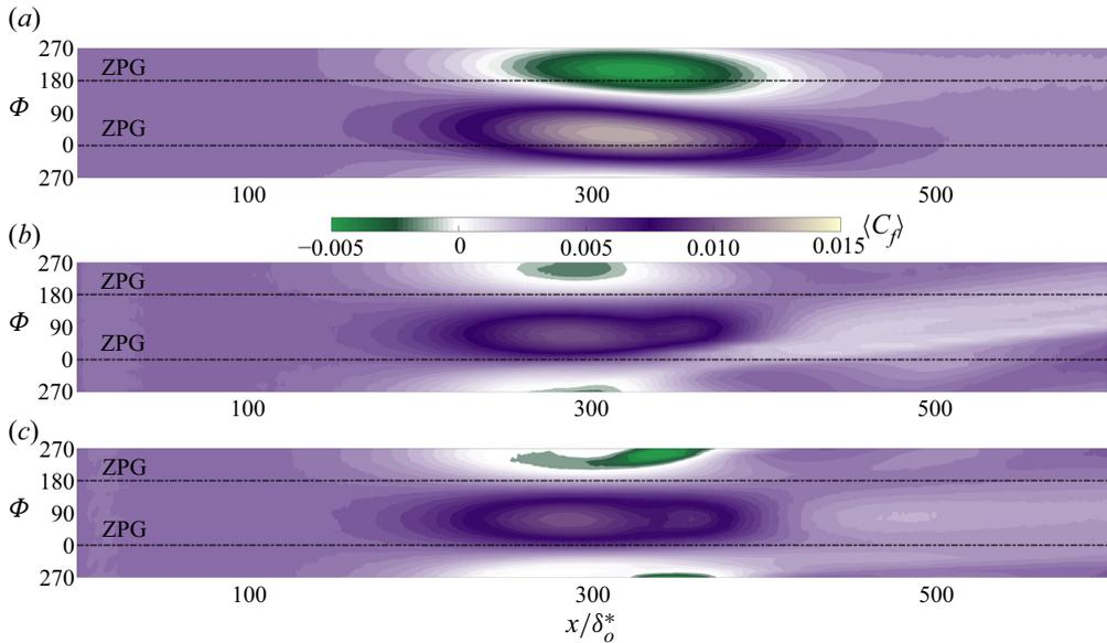
Figure 15. Contours of phase-averaged skin-friction coefficient  $\langle C_f \rangle$  as a function of the streamwise direction  $x$  and phase  $\Phi$ . Black dashed-dotted lines denote the ZPG phases: (a)  $k = 10$ ; (b)  $k = 1$ ; (c)  $k = 0.2$ .
