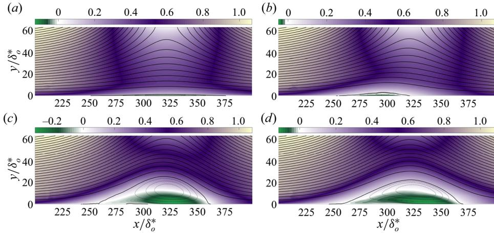
Figure 12. Contours of phase-averaged streamwise velocity  $\langle u \rangle$  for the phase  $\Phi = 270^\circ$ : (a)  $k = 10$ ; (b)  $k = 1$ ; (c)  $k = 0.2$ ; (d) steady calculation (SC-1). Solid and dashed lines denote positive and negative values of the streamfunction, respectively.
