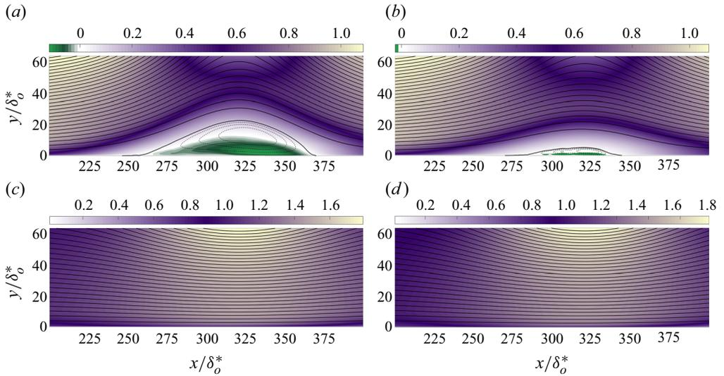
Figure 5. Contours of streamwise time-averaged velocity  $\bar{u}$  for the steady calculations corresponding to the following phases: (a) SC-1  $\Phi = 270^\circ$ ; (b) SC-2  $\Phi = 306^\circ$ ; (c) SC-4  $\Phi = 54^\circ$ ; (d) SC-5  $\Phi = 90^\circ$ . Solid and dashed lines denote positive and negative values of the streamfunction, respectively.
