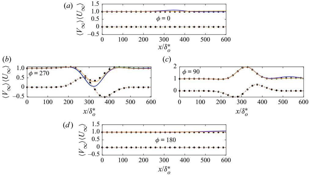
Figure 8. Profiles of free-stream streamwise  $\langle U_\infty \rangle$  and wall-normal  $\langle V_\infty \rangle$  phase-averaged velocity. Only the main four phases of the cycle are shown (see figure 4). Symbols denote the steady calculations, lines represent dynamic results at different reduced frequencies  $k$ . Solid lines  $U_\infty$ , dashed lines  $V_\infty$ . Colours are as follows: ● steady case; green lines,  $k = 10$ ; blue lines,  $k = 1$ ; orange lines,  $k = 0.2$ .
