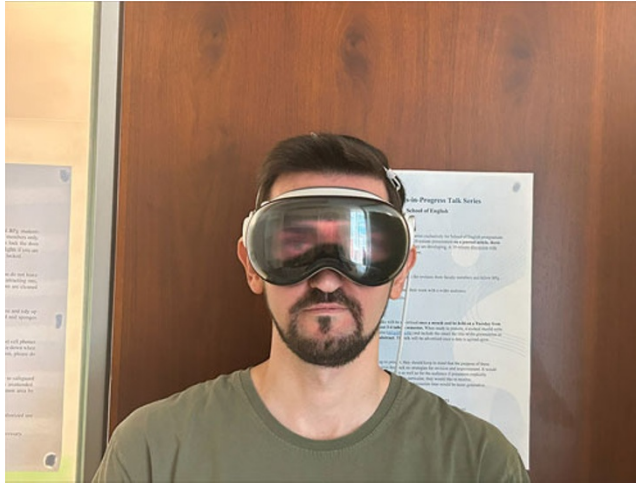
Figure 5. Virtual eyes projected onto the external screens of the Vision Pro (photo by Ruyu Yan).
