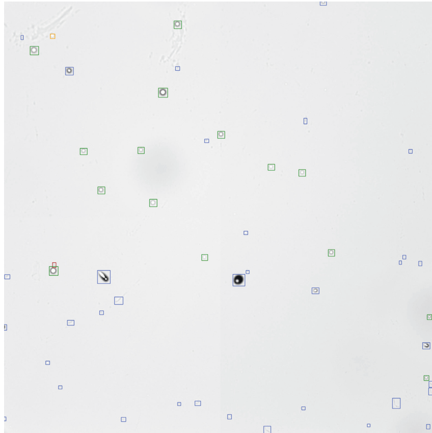
FIGURE 3: An example of FAINE tagging signs inside a CR-39 image. Green squares indicate true positives, blue squares indicate true negatives, red squares indicate false positives, and orange squares indicate false negatives.
