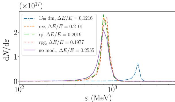
FIGURE 2. Kinetic energy of ions for different targets from figure 1 with modulation parameters,  $k_m = 2$  and  $a_m = 0.25$  at  $t/\tau_L = 440$ . The other parameters are  $a_0 = 150$ ,  $n_e = 250n_c$  and  $d = 1.0\lambda_L$  in each case. The y axis represents the proton numbers,  $N$  per unit length. Moving window velocities are  $v_{\text{mov}} = 0.8c$  for dm target, and  $v_{\text{mov}} = 0.75c$  for surface modulated and flat targets.
