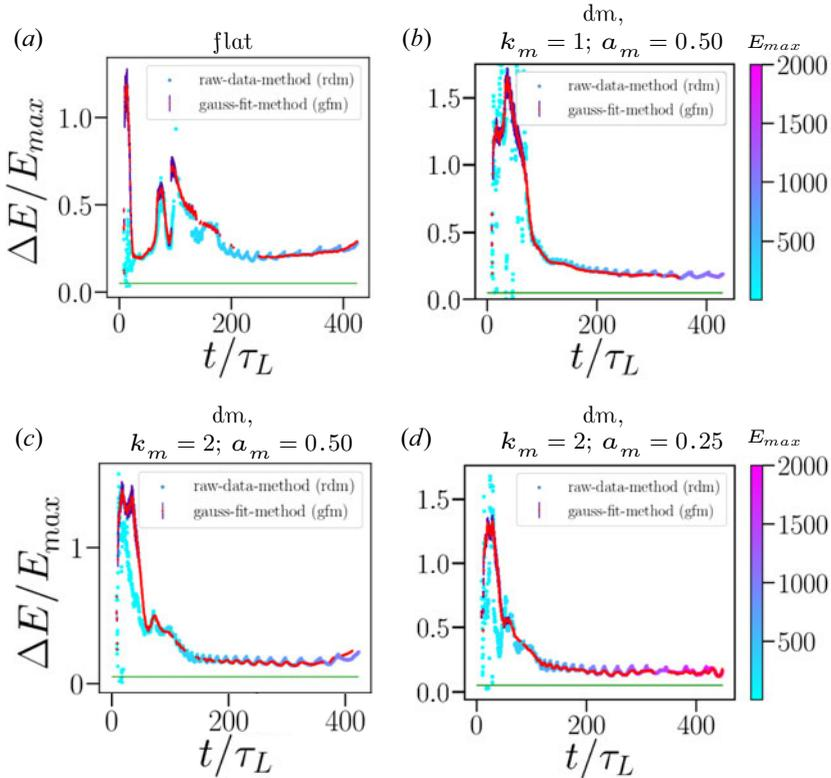
FIGURE 4. Evolution of the  $\Delta E/E_{\max}$  with time. The colourbar denotes the  $E_{\max}$  (in MeV) in each case. (a) The flat target, (b) dm with  $k_m = 1$ ,  $a_m = 0.50$ , (c)  $k_m = 2$ ,  $a_m = 0.50$  and (d)  $k_m = 2$ ,  $a_m = 0.25$ . The target width is  $d = 1.0\lambda_L$  in each case. The green line is the sought limit of  $\Delta E/E_{\max} = 0.05$  (5%). The other parameters are the same as in figure 2.
