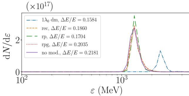
FIGURE 7. Kinetic energy of ions for different targets with modulation parameters  $k_m = 2$ ,  $a_m = 0.25$ , at  $t/\tau_L = 314$  with RR ( $a_0 = 250$ ). The target width is  $d = 1.0\lambda_L$  in each case. Moving window velocities are  $v_{\text{mov}} = 0.84c$  for dm target, and  $v_{\text{mov}} = 0.8c$  for surface modulated and flat targets.
