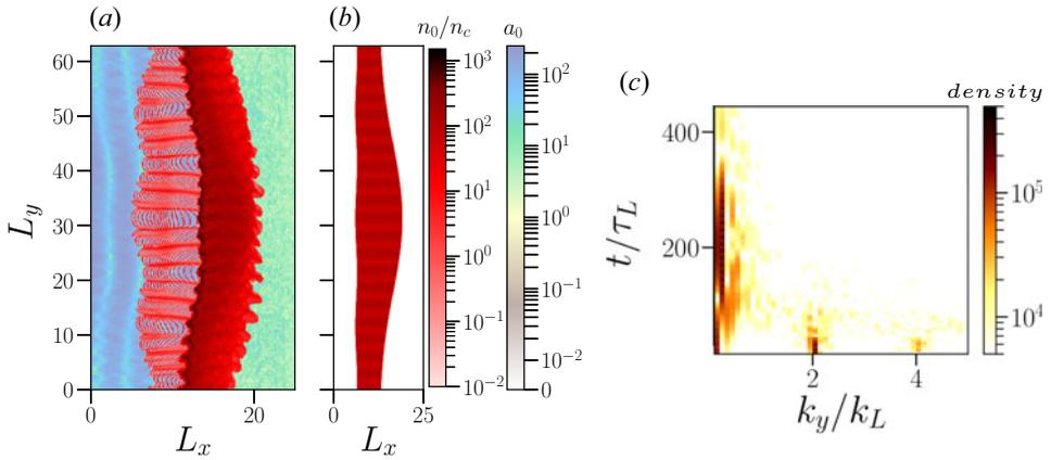
FIGURE 15. Proton density of a target with dm-rpg. The laser pulse has a spatial Gaussian profile with  $a_0 = 150$ . Panel (a) is at  $t/\tau_L = 40$ , while the initial profile at  $t/\tau_L = 0$  is shown in (b). (c) Time development of the FFT of the proton density. Modulation parameters are  $a_m = 0.25$ ,  $k_m = 2$ , and the target widths varies between  $d = 2.0\lambda_L$  and  $d = 1.0\lambda_L$  (see (3.11)). Moving window velocity is  $v_{\text{mov}} = 0.8 c$ .
