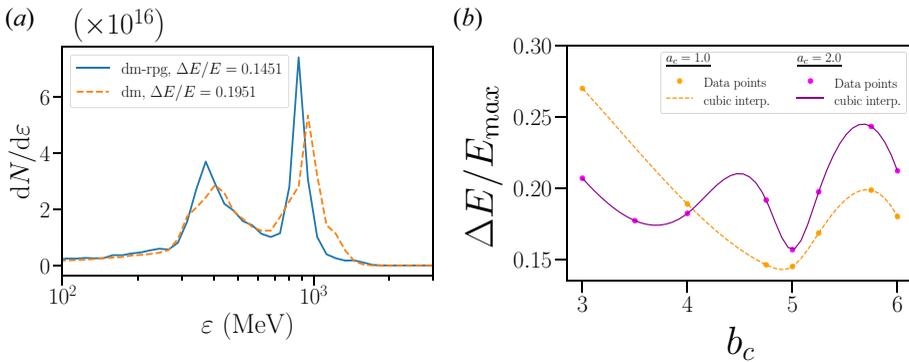
FIGURE 16. (a) Proton energy spectra corresponding to figure 15(a) at  $t/\tau_L = 280$  for  $a_c = 1.0$ ,  $b_c = 5.0$ . (b) Cubic interpolation of  $\Delta E/E_{\text{max}}$  with  $b_c$  and with  $a_c = 1.0$  and  $a_c = 2.0$ . The other parameters are  $a_m = 0.25$ ,  $k_m = 2$ ,  $a_0 = 150$ .
