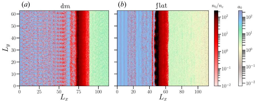
FIGURE 3. Evolution of the ion density and the normalised laser electric field  $a_0$  for (a) a density modulated target ( $k_m = 2$ ,  $a_m = 0.25$ ) and (b) the flat target, for  $a_0 = 150$ . Both targets have  $d = 1.0\lambda_L$  width. The results are shown at  $t/\tau_L = 144$ . The other parameters are the same as in figure 2.
