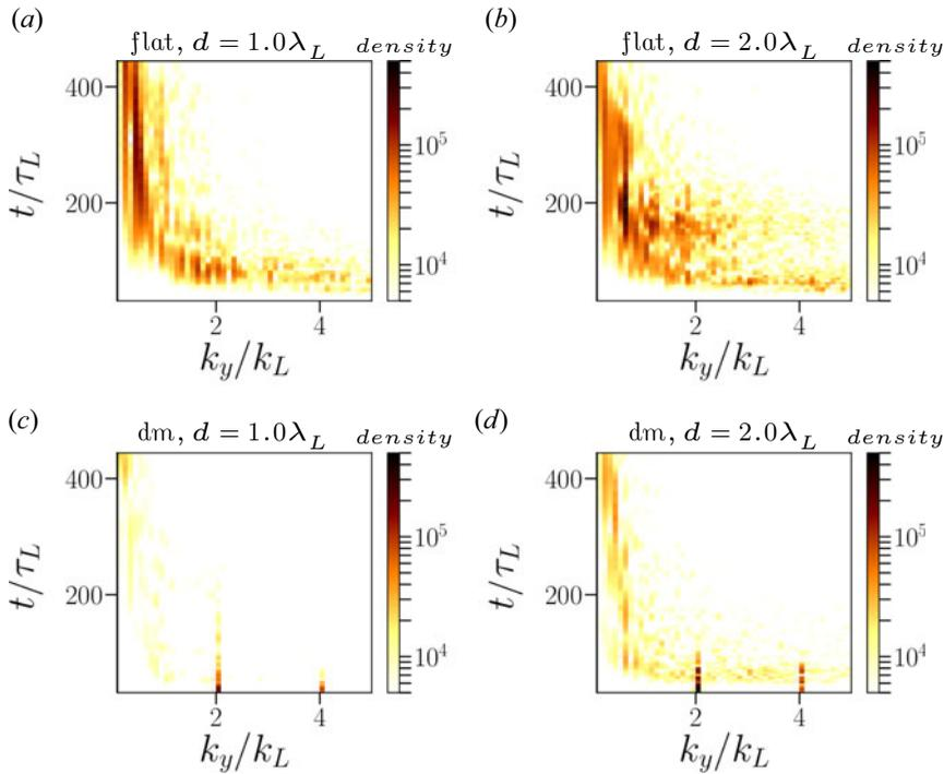
FIGURE 14. Time development of the FFT of ion density oscillations including RR force for the flat target (a,b) and the density modulated target (c,d) at  $a_0 = 350$ . Panels (a,c) and (b,d) correspond to the target widths of  $d = 1.0\lambda_L$  and  $d = 2.0\lambda_L$ , respectively. The modulation parameters are  $a_m = 0.50$ ,  $k_m = 2$ .
