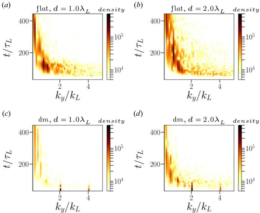
FIGURE 13. Time development of the FFT of ion density oscillations including RR force for the flat target (*a,b*) and the density modulated target (*c,d*) at  $a_0 = 250$ . Panels (*a,c*) and (*b,d*) correspond to the target widths of  $d = 1.0\lambda_L$  and  $d = 2.0\lambda_L$ , respectively. The modulation parameters are  $a_m = 0.50$ ,  $k_m = 2$ .
