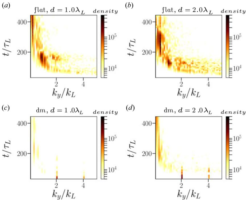
FIGURE 12. Time development ( $t/\tau_L$ ) of the FFT of the ion density of a flat target ( $a,b$ ), and for a density modulated target ( $c,d$ ) with the normalised wavevector  $k_y/k_L$ . Panels ( $a,c$ ) and ( $b,d$ ) are for  $d = 1.0\lambda_L$  and  $d = 2.0\lambda_L$  target widths in respective cases. The modulation parameters are  $a_m = 0.25$ ,  $k_m = 2$ .
