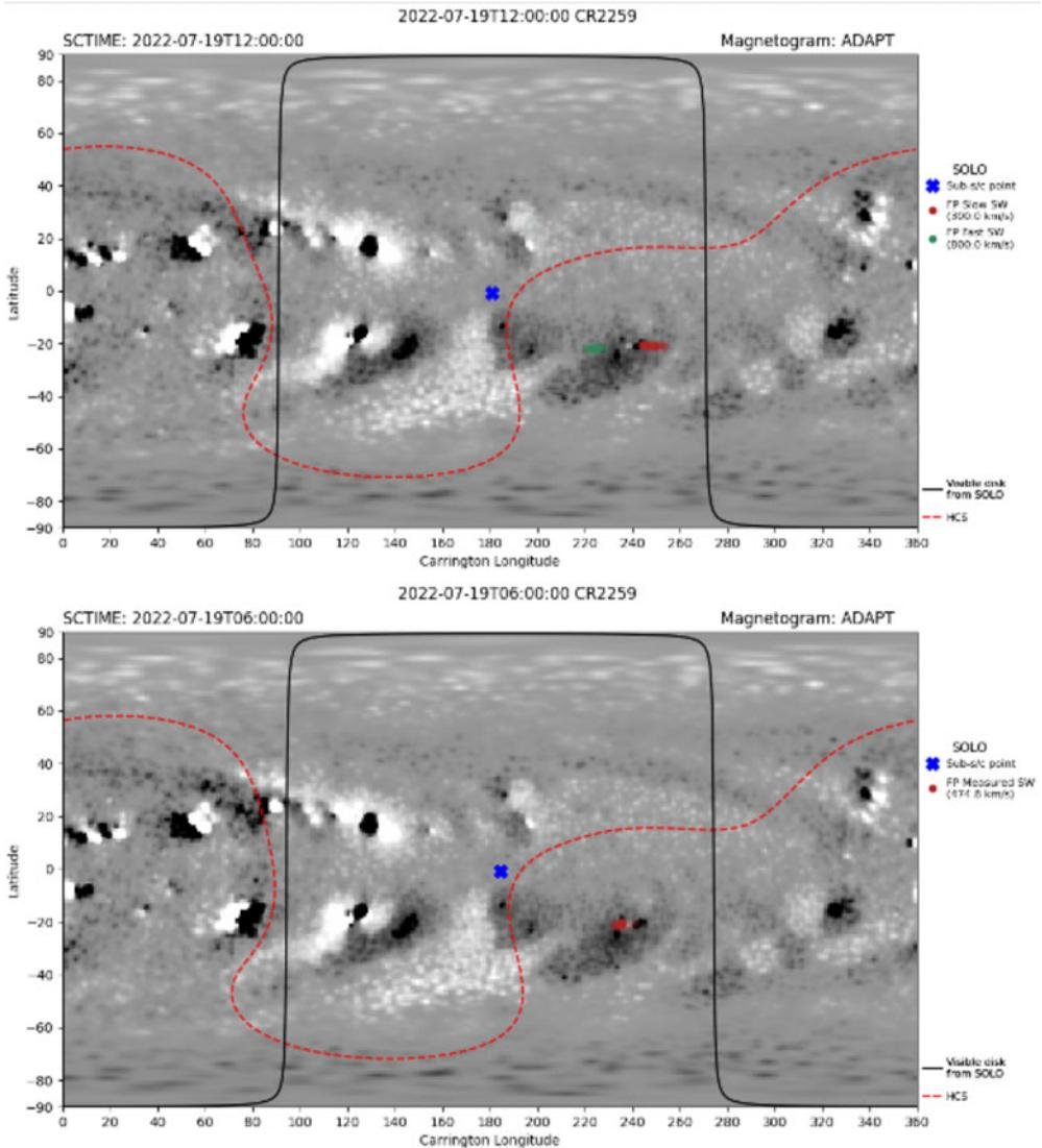
**Figure 3.** Examples of a connectivity map estimated without (top panel) and with (bottom) the integration of the measured solar wind speed from the SWA/PAS LLD. The red line is the HCS while the green and red dots represent the fast and slow wind connection points, respectively.
