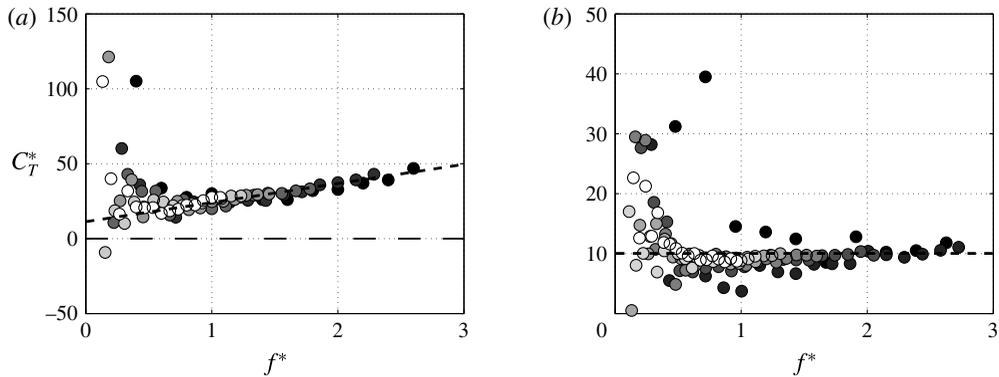
FIGURE 7. Newly non-dimensionalized thrust as a function of reduced frequency for (a) heaving and (b) pitching. Equations (6.2) and (6.3) are shown by the dashed lines. Colours are the same as in figures 3 and 5.
