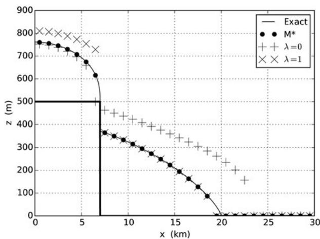
Fig. 8. Results from  $M^*$  method, and its upwinding variations with different  $\lambda$  values in formula (30), compared with the bedrock-step exact solution, on a  $\Delta x = 1000$  m grid. The bedrock itself is shown with a thick solid line.
