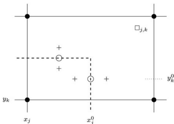
**Fig. 4.** On element  $\square_{j,k}$ , when computing the flux at quadrature points (circles), upwinding of the flux term  $\tilde{\mathbf{q}} = \mathbf{W}H^{n+2}$  evaluates the thicknesses  $H$  at locations shown with ‘+’, one-quarter of the way to the element boundary.
