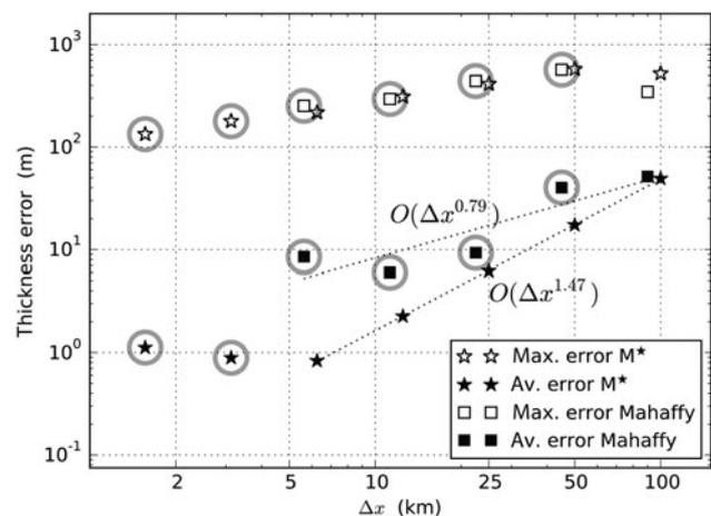
Fig. 6. Average and maximum error under grid refinement using the dome exact solution, for the  $M^*$  (stars) and classical Mahaffy (squares) methods. Gray circles indicate runs where the Newton method diverged before the last  $\epsilon_{12} = 0$  continuation stage.
