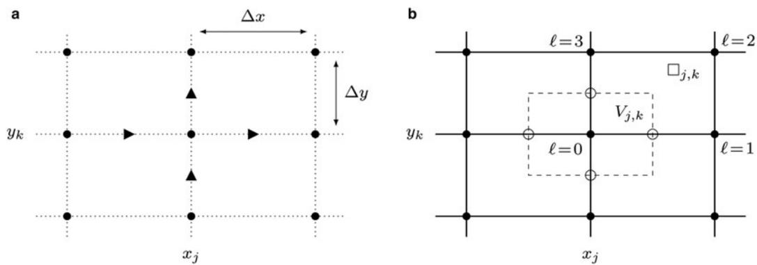
**Fig. 1.** (a) A structured FD grid with regular (dots) and staggered (triangles) points. (b) The same grid as an FVE grid with rectangular elements  $\square_{j,k}$  (solid), nodes (dots), a dual rectangular control volume  $V_{j,k}$  (dashed) and Mahaffy's flux-evaluation locations (circles). The corners of element  $\square_{j,k}$  are locally indexed by  $\ell$ .
