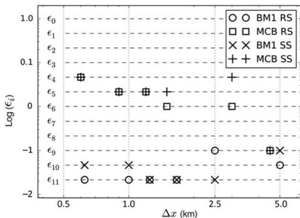
**Fig. 9.** Smallest successful value of  $\epsilon_i$  for which the Newton iteration converges on the steady-state problem; lower is better. Different bed data sources (BM1 or MCB) and complementarity-problem solvers (RS or SS) are compared.
