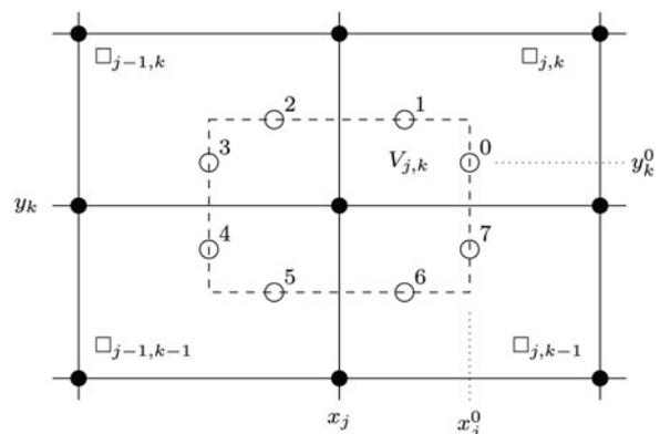
Fig. 3. For Eqn (26) we evaluate  $\mathbf{q}^h(x, y)$  at eight quadrature points (numbered circles) along  $\partial V_{j,k}$  (dashed).
